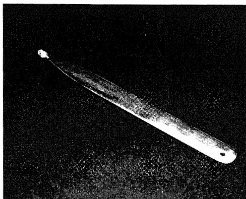
Fig. 1-4 Tapping inspection stick
