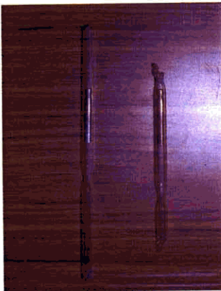
Fig. 2.3-2 Alloy specimens enclosed in silica glass tubes under 1 \times 10^{-4} Pa after dehydration.
