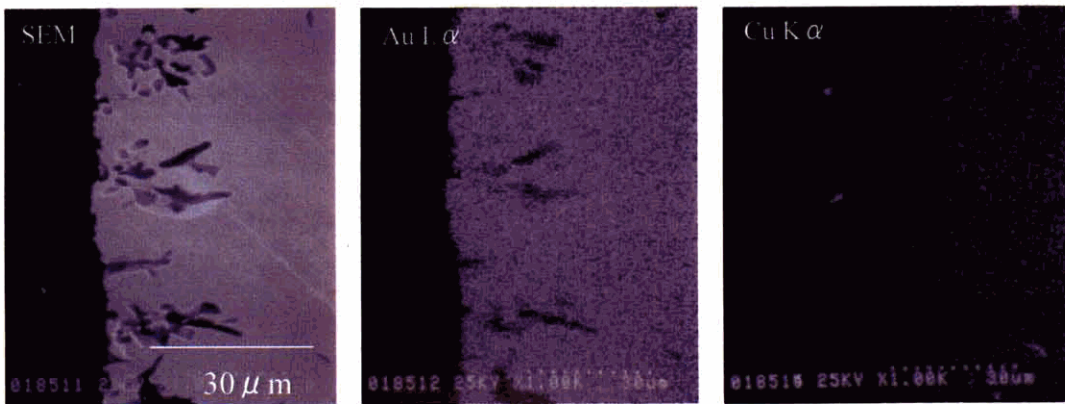
Fig. 6.1-3 Secondary electron image (a) and X-ray images of Au L α (b) and Cu K α (c) obtained from a specimen treated by oxidation and pickling.
