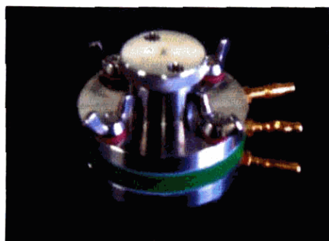
Fig. 5-2-2 Photograph of the electrochemical cell.
