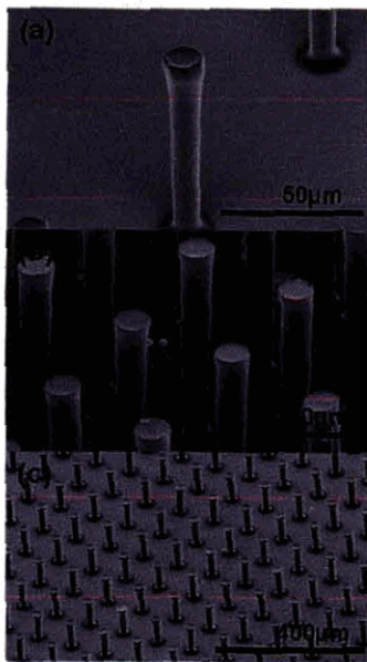
Fig. 7-8 Typical SU-8 post arrays after pyrolysis on different substrate with different feature. (C. Wang, et al., Electrochem. Solid-State Lett. , 7-11, A435 (2004).)
