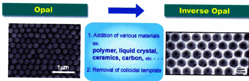
Fig. 1-3-22 Outline of procedure for the inverse opal materials prepared by opal template.
