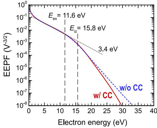
FIG. 5. Normalized EEPFs in the entire plasma area based on the inductive model (w/o CC) and the hybrid model (w/ CC) under the same conditions as those in Fig. 3. Here,  $E_{ex}$  and  $E_{iz}$  are the excitation and ionization threshold energies, respectively.
