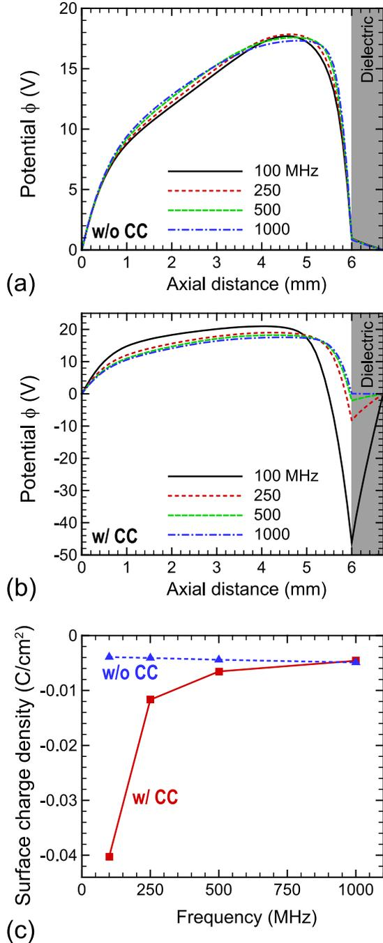
FIG. 7. Axial distributions of  $\phi$  at the innermost coil ( $r=1.3$  mm) in the mICP based on (a) the inductive model (w/o CC) and (b) the hybrid model (w/ CC); (c) the surface charge density on the dielectric window at  $r=1.3$  mm as a function of rf frequency under the same conditions as those in Fig. 6.
