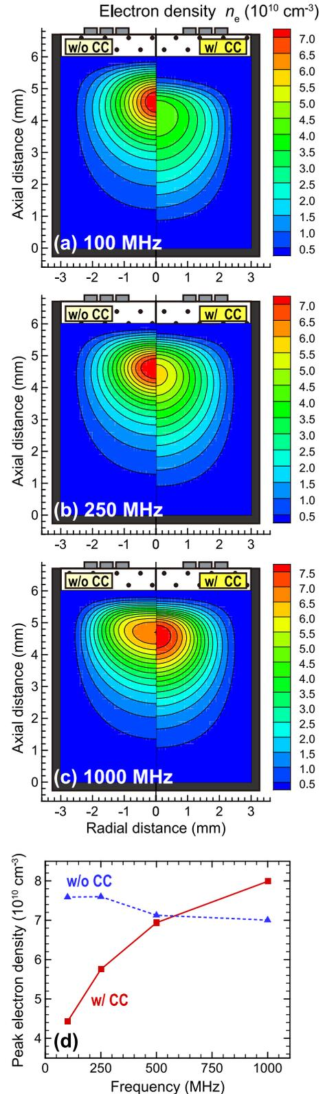
FIG. 6. Two-dimensional distributions of the time-averaged electron density  $n_e$  in the mICP based on the inductive model (left, w/o CC) and the hybrid model (right, w/ CC) for  $f=(a) 100,$  (b) 250, and (c) 1000 MHz; (d) the peak  $n_e$  as a function of rf frequency, calculated at  $p=500$  mTorr and  $P_{abs}=10$  mW.
