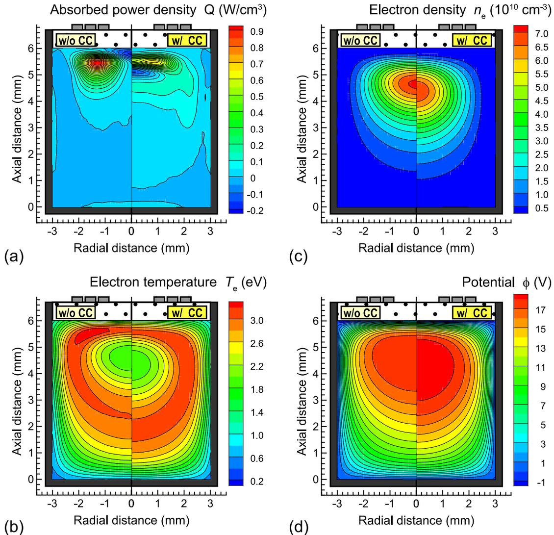
FIG. 3. Two-dimensional distributions of the time-averaged (a) absorbed power density  $Q$ , (b) electron temperature  $T_e$ , (c) electron density  $n_e$ , and (d) potential  $\phi$  in the mICP based on the inductive model (left, w/o CC) and the hybrid model (right, w/ CC), calculated at the Ar gas pressure  $p = 500$  mTorr, rf frequency  $f = 500$  MHz, and absorbed power  $P_{abs} = 10$  mW as a base case condition.
