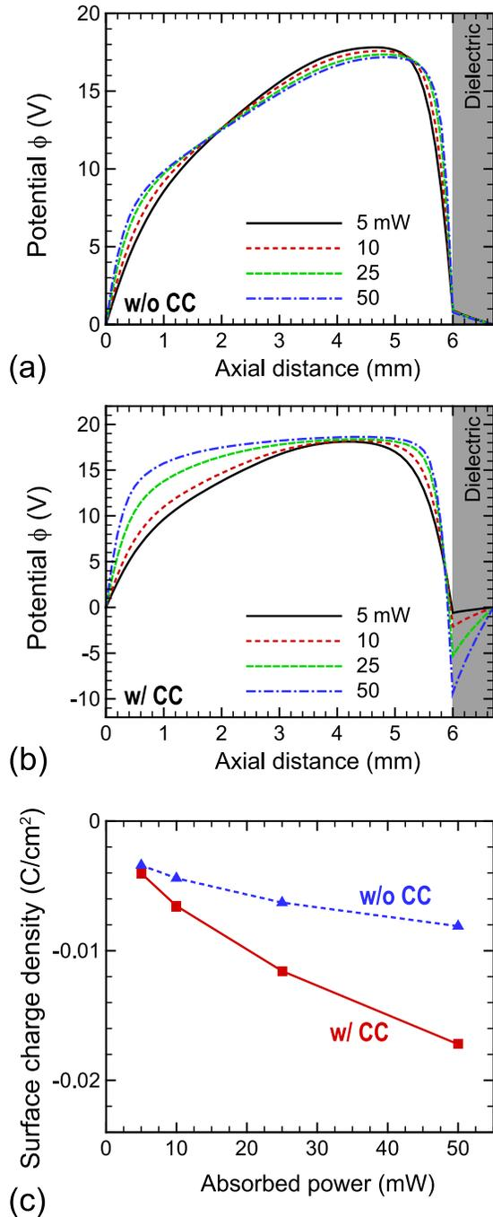
FIG. 10. Axial distributions of  $\phi$  at the innermost coil ( $r=1.3$  mm) in the mICP based on (a) the inductive model (w/o CC) and (b) the hybrid model (w/ CC); (c) the surface charge density on the dielectric window at  $r=1.3$  mm as a function of absorbed power under the same conditions as those in Fig. 9.
