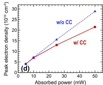
FIG. 9. Two-dimensional distributions of the time-averaged electron density  $n_e$  in the mICP based on the inductive model (left, w/o CC) and the hybrid model (right, w/ CC) for  $P_{abs} =$  (a) 5, (b) 25, and (c) 50 mW; (d) the peak  $n_e$  as a function of absorbed power, calculated at  $p = 500$  mTorr and  $f = 500$  MHz.
