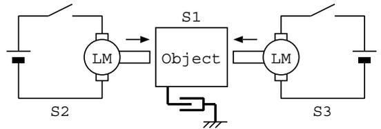
Fig. 8. Decentralized actuation system
