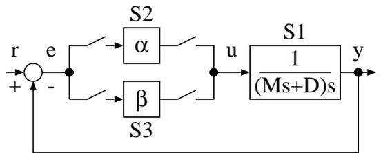
Fig. 9. Variable structure system with sliding mode
