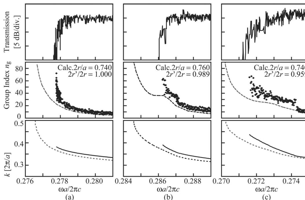
Fig. 3. Measured transmission spectrum,  $n_g$  characteristics, and band diagram experimentally evaluated for  $2r/a=0.65$  (solid curve) and calculated for the parameters in the figures (dashed curve).  $2r'/2r$  is (a) 1.00, (b) 0.89, (c) 0.86.
