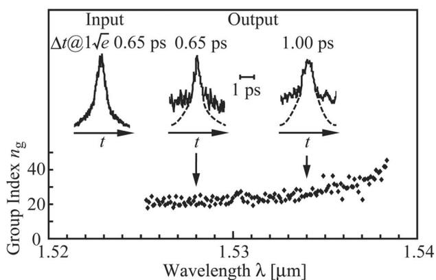
Fig. 4. Group index  $n_g$  characteristics for another sample ( $2r/a=0.64$ ,  $2r'/2r=0.84$ ) showing LVL characteristics and autocorrelation traces of input and output optical pulses.
