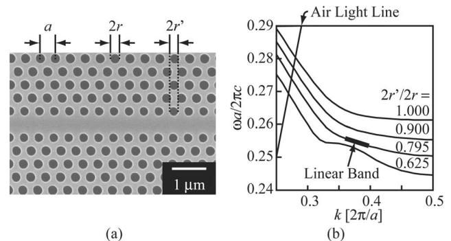
Fig. 1. Device structure and photonic band. (a) Top view of LVL PCW fabricated on SOI substrate. (b) Photonic band of the main propagation mode of PCW for  $2r/a=0.667$ .  $2r'/2r$  is taken as a parameter.
