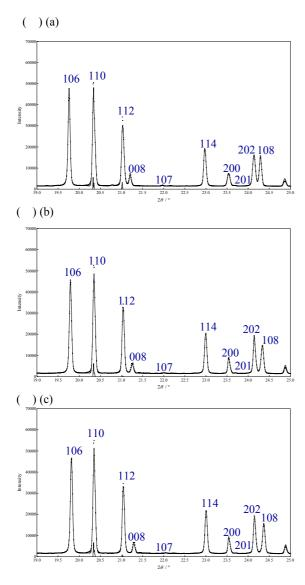
Fig. 2. Rietveld fitting pattern of synchrotron radiation powder X-ray data at (a)300K, (b)200K and (c)100K for ( ) x=0.81.
