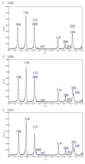
Fig. 1. Rietveld fitting pattern of synchrotron radiation powder X-ray data at (a)300K, (b)200K and (c)100K for ( ) x=0.75.
