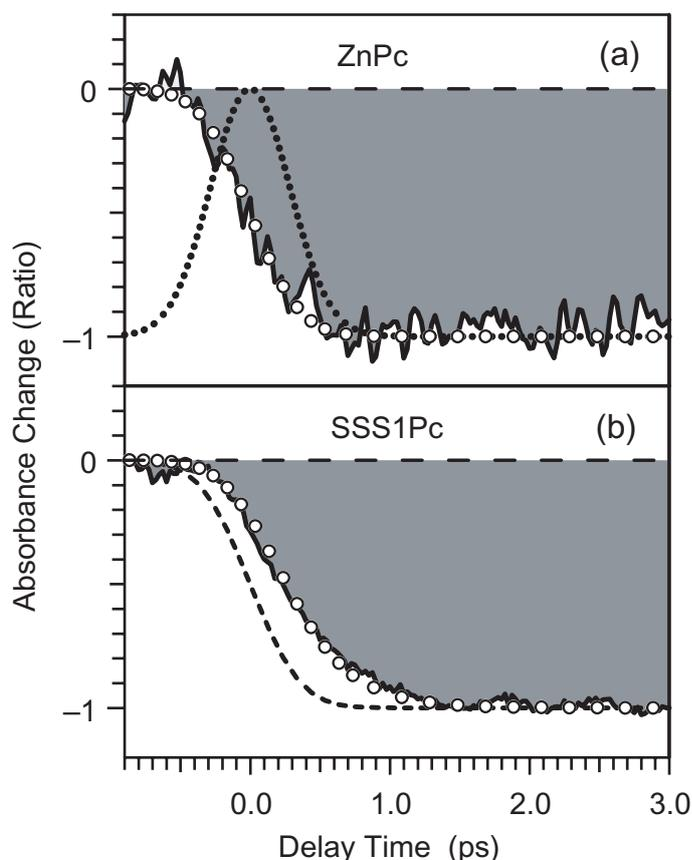
**Figure 7.** Ultrafast responses of bleaching of the Q-absorption band for (a) ZnPc and (b) SSS1Pc. The dotted line in (a) indicates the temporal profile of the instrument response function. Dark-grey regions indicate the temporal profiles of the Q-band bleachings. Fitted results with respective rising components are plotted using open circles. The dashed line in (b) is a visual guide and indicates the fitted result for ZnPc (open circles in (a)).
