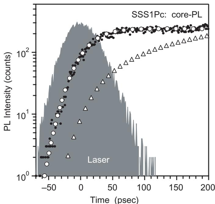
**Figure 5.** Rising behaviour of the PL for the core in SSS1Pc (filled dots). Grey profiles are observed temporal profiles of the excitation light pulses. Profiles indicated by open circles and triangles are simulation results using values for the rising time constant  $\tau_{\text{rise}}$  of 0.02 ns and 1.5 ns ( $\tau_{\text{Ant}}(\text{RT})$ ), respectively.
