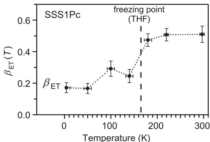
**Figure 11.** Filled circles: temperature dependence of the ET quantum efficiency  $\beta_{ET}$  in SSS1Pc. The vertical broken line indicates the FP of the solvent (THF).
