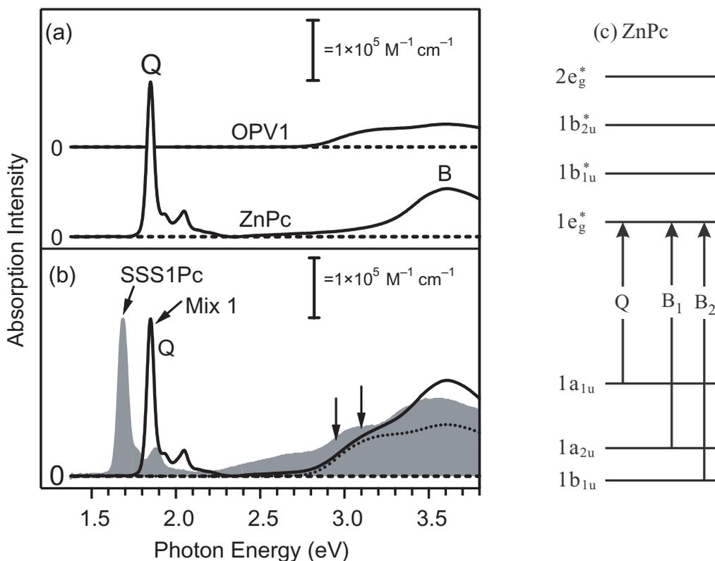
**Figure 2.** (a) Absorption spectra of the component molecules ZnPc and OPV1. (b) Absorption spectra of SSS1Pc (grey region) and Mix 1 (solid line) solutions. Arrows indicate the excitation energy for PL and pump-probe measurements. (c) Energy diagram of MOs for ZnPc (figure 8 in [25]) having  $D_{4h}$  symmetry. MOs lower than  $1b_{1u}$  and MOs higher than  $2e_g^*$  are omitted. Solid arrows indicate the optical transitions of the respective absorption bands (Q, Soret:  $B_1$ ,  $B_2$ ).
