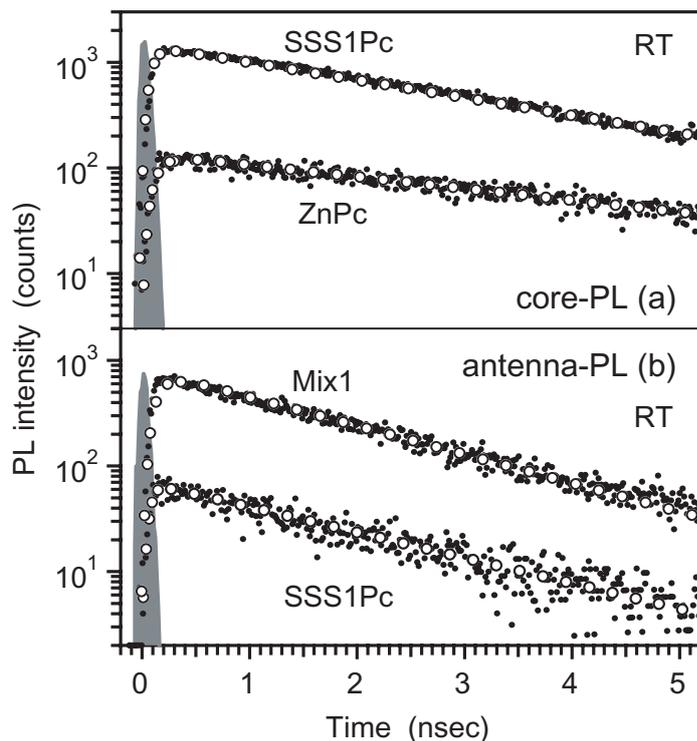
**Figure 4.** Decay profiles of PL intensities (a) of the core and (b) of the antenna (filled dots). Grey profiles are the measured temporal profiles of the excitation light pulse. Profiles indicated by open circles are the fitting results of deconvolution analysis.
