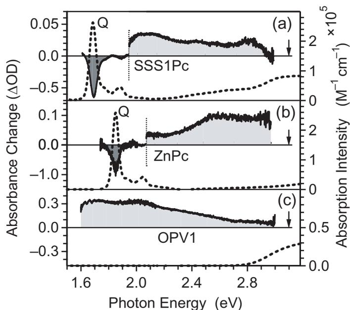
**Figure 6.** Transient absorption change spectra for (a) SSS1Pc, (b) ZnPc and (c) OPV1. Grey spectra indicate transient absorption change spectra at 3 ps (2.5–3.5 ps) after photoexcitation. Dashed lines show the normal absorption spectra without pumping. Dark and light-grey areas denote bleaching of absorption and induced absorption, respectively. The arrows indicate the energy of the pump laser. The increments of the vertical scale are increased by a factor of 10 in the vicinity of the Q-band.
