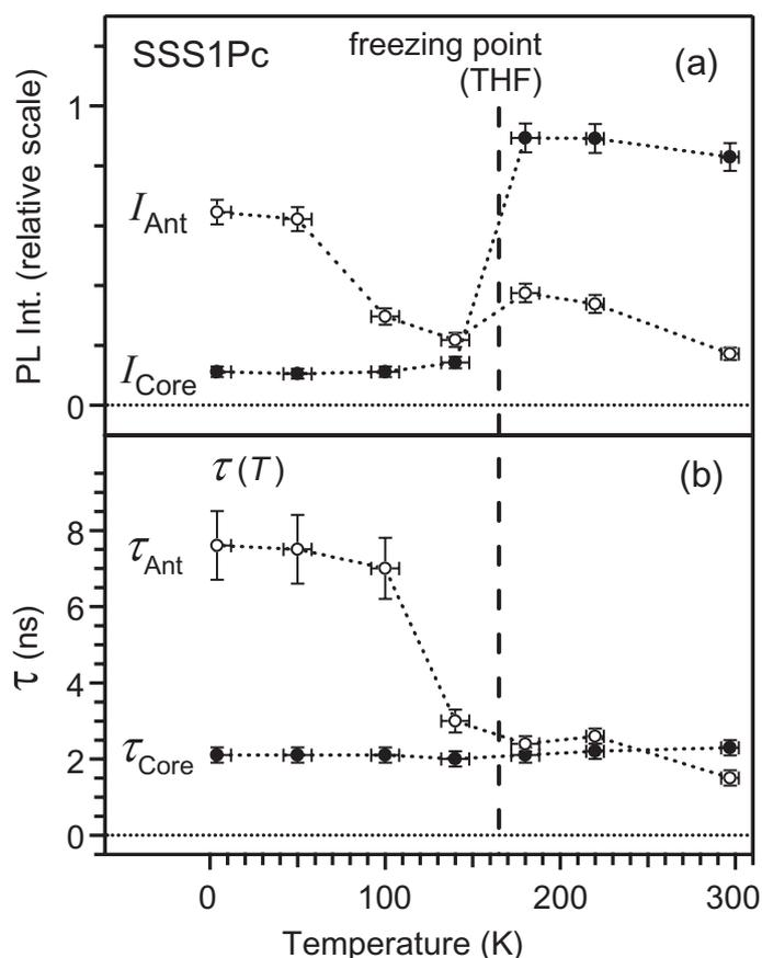
**Figure 9.** (a) Temperature dependence of the PL intensities of the core  $I_{\text{Core}}$  (●) and of the antennas  $I_{\text{Ant}}$  (○). (b) Temperature dependence of the decay time constants for the PL of the core  $\tau_{\text{Core}}$  (●) and for the PL of the antennas  $\tau_{\text{Ant}}$  (○). The vertical broken line indicates the freezing point of the solvent THF. The magnitude of the error bar indicate the error width of  $1\sigma$ .
