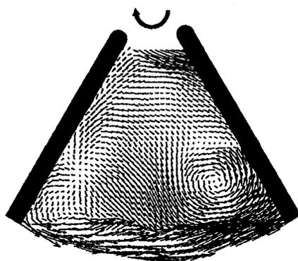
Fig. 3 Measured relative velocity vectors of a Semi-open impeller S1 ( $N_s=100$ ,  $Q/Q_0=0.25$ )
