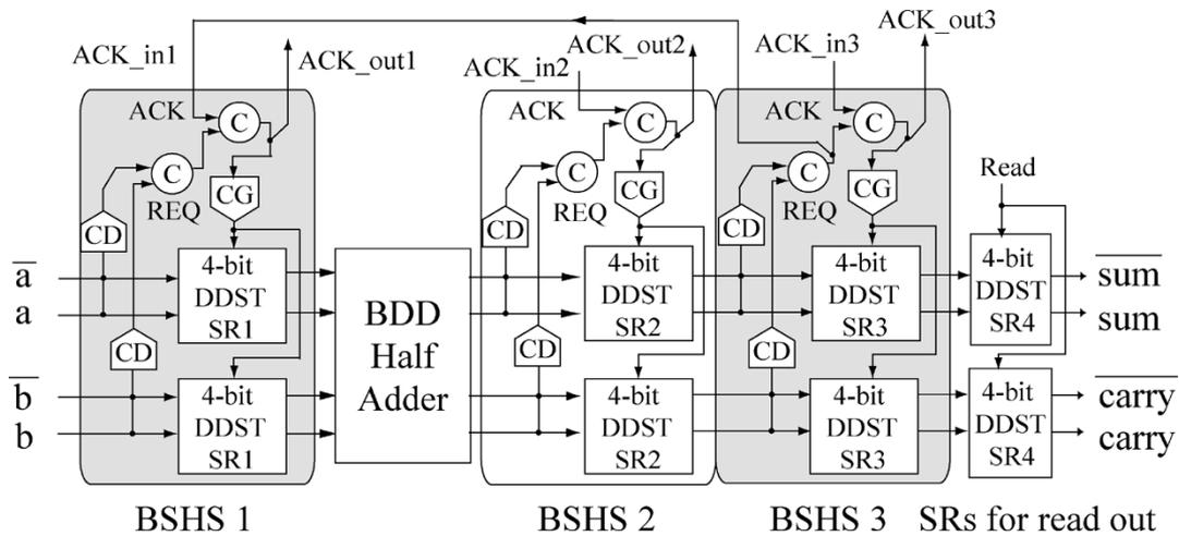
Fig. 3. A test system for a two-input bit-serial handshaking system, which is composed of three stages of the BSBS modules, one BDD half adder and two shift registers for read out.
