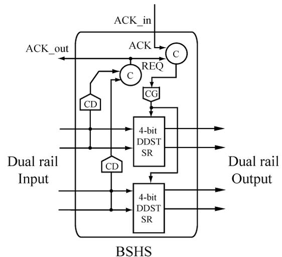
Fig. 2. A block diagram of a two-input BSHS module.
