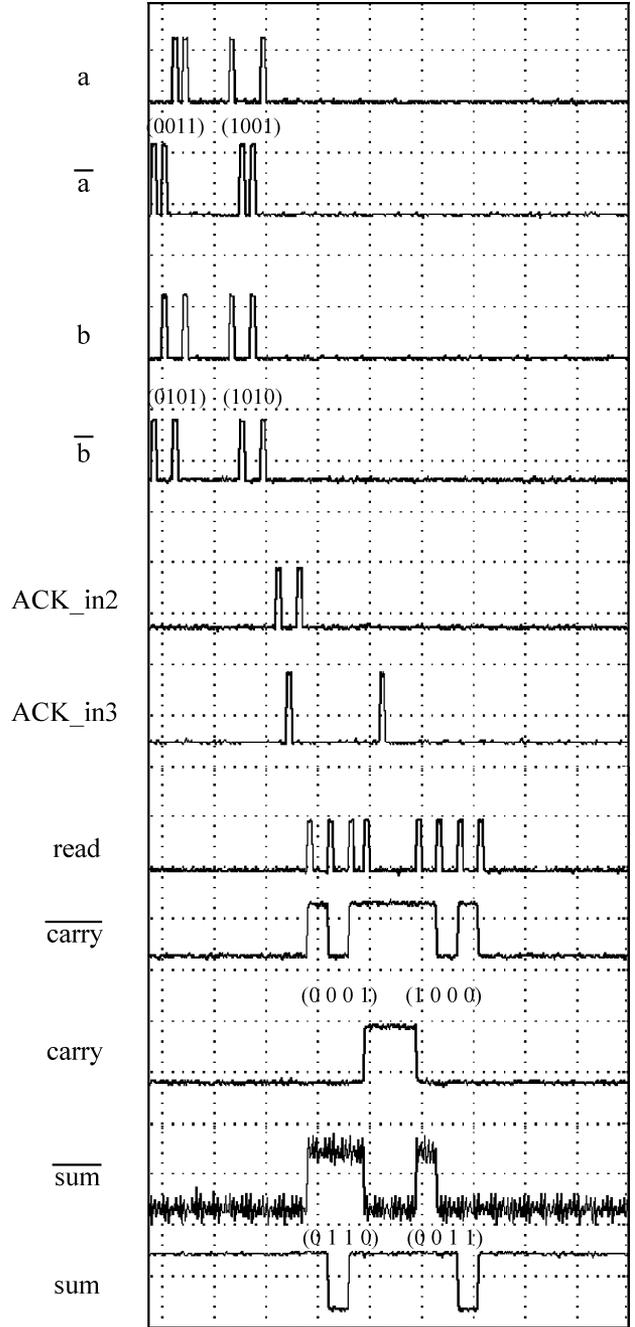
Fig. 5. Test results of the BSHS half adder system shown in Fig. 3. The scales of y-axis for the input (a, a\_bar, b, b\_bar, ACK\_in2, ACK\_in3, and read) is 20 mV/div and the scales for the output (carry\_bar, carry, sum\_bar, and sum) is 200  $\mu\text{V}/\text{div}$ . The rising edges in the input signals correspond to the inputs of SFQ pulses, and the transitions in the output signals are the output of SFQ pulses. The scale of x-axis is 10 ns/div.
