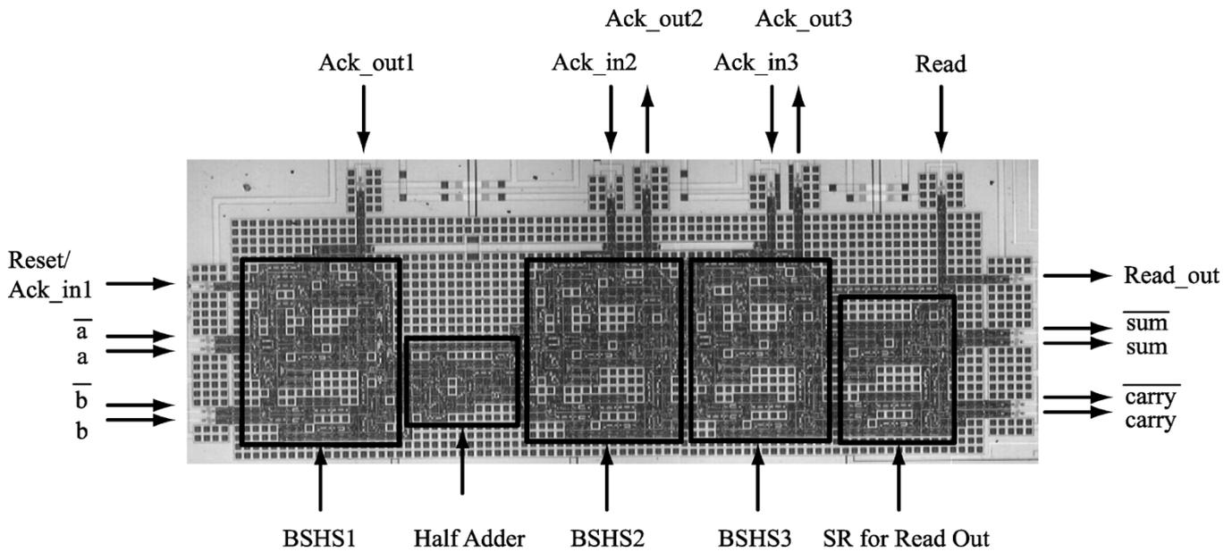
Fig. 4. A photomicrograph of the test system.
