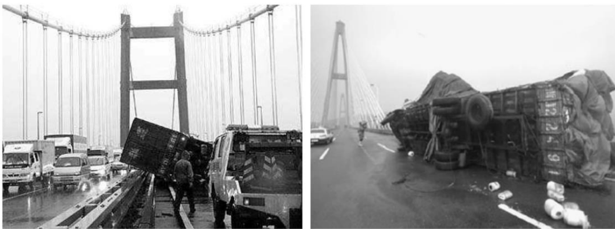
Figure 1.1 Wind-induced traffic accidents (Zhang et al., 2020)
