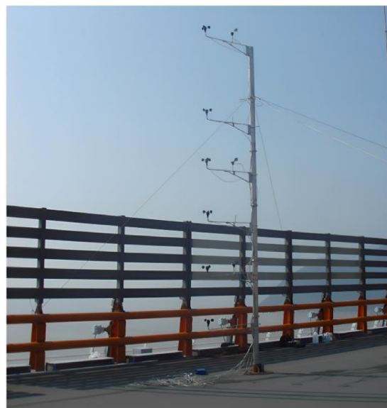
Figure 1.2 Wind barrier installed on the handrail with on-site wind speed measurement (Yang et al., 2022)
