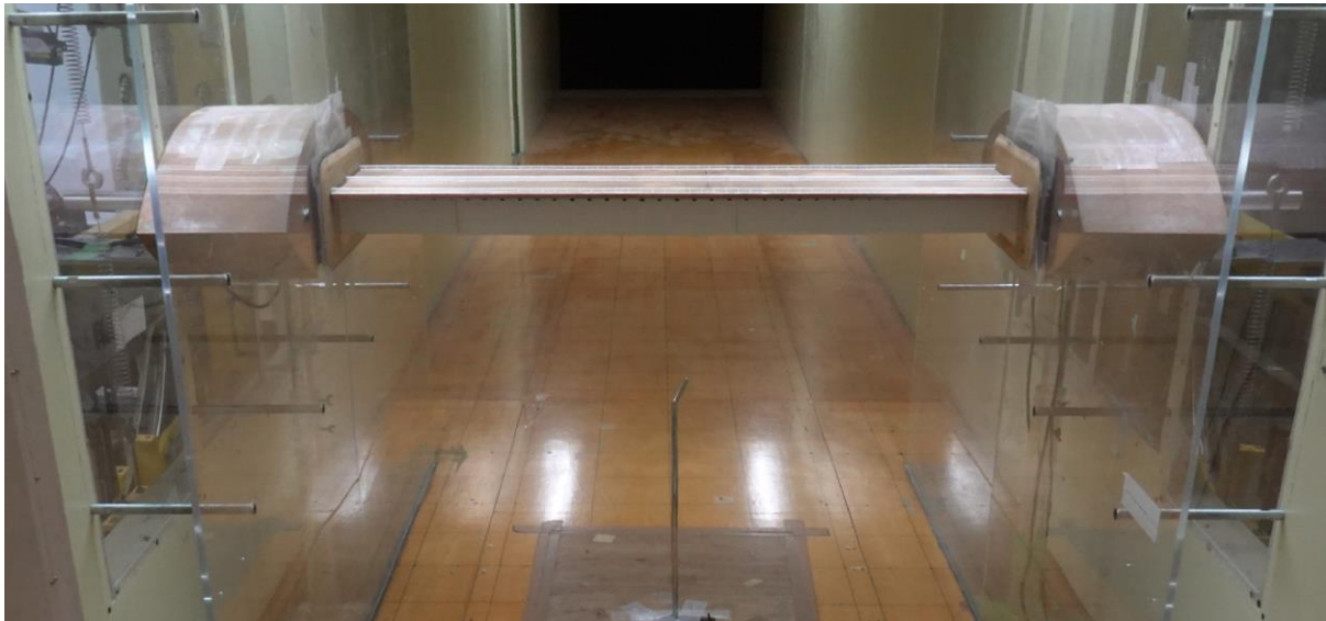
Figure 3.4 A sectional model in a wind tunnel for aerodynamic force coefficient measurement
