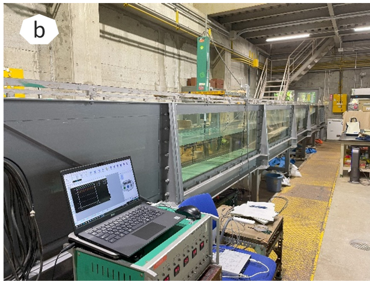
Figure A.7: Calibration process for pressure transducers (PTs): (a) PTs with the elevator and (b) data recording software (DCS-100A).
