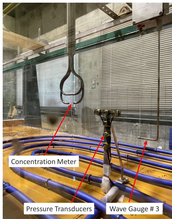
Figure A.4: Instrumental setup at cross-shore location of x = 200 cm: Pressure transducers, Concentration meter and Wave gauge.
