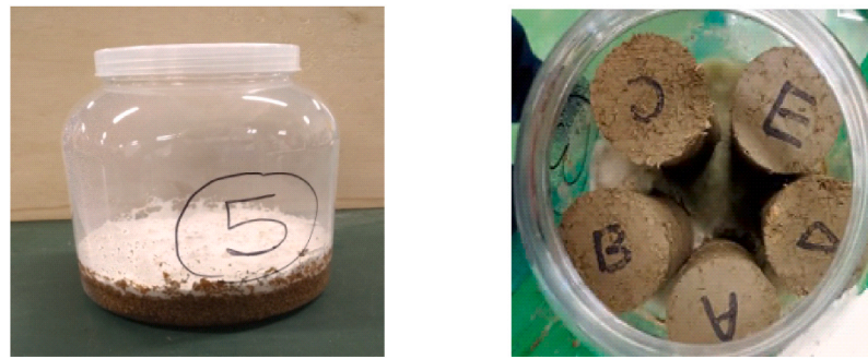
(a) Kawaratake fungal mycelia in the incubator (b) Treated clay specimens in the incubator
