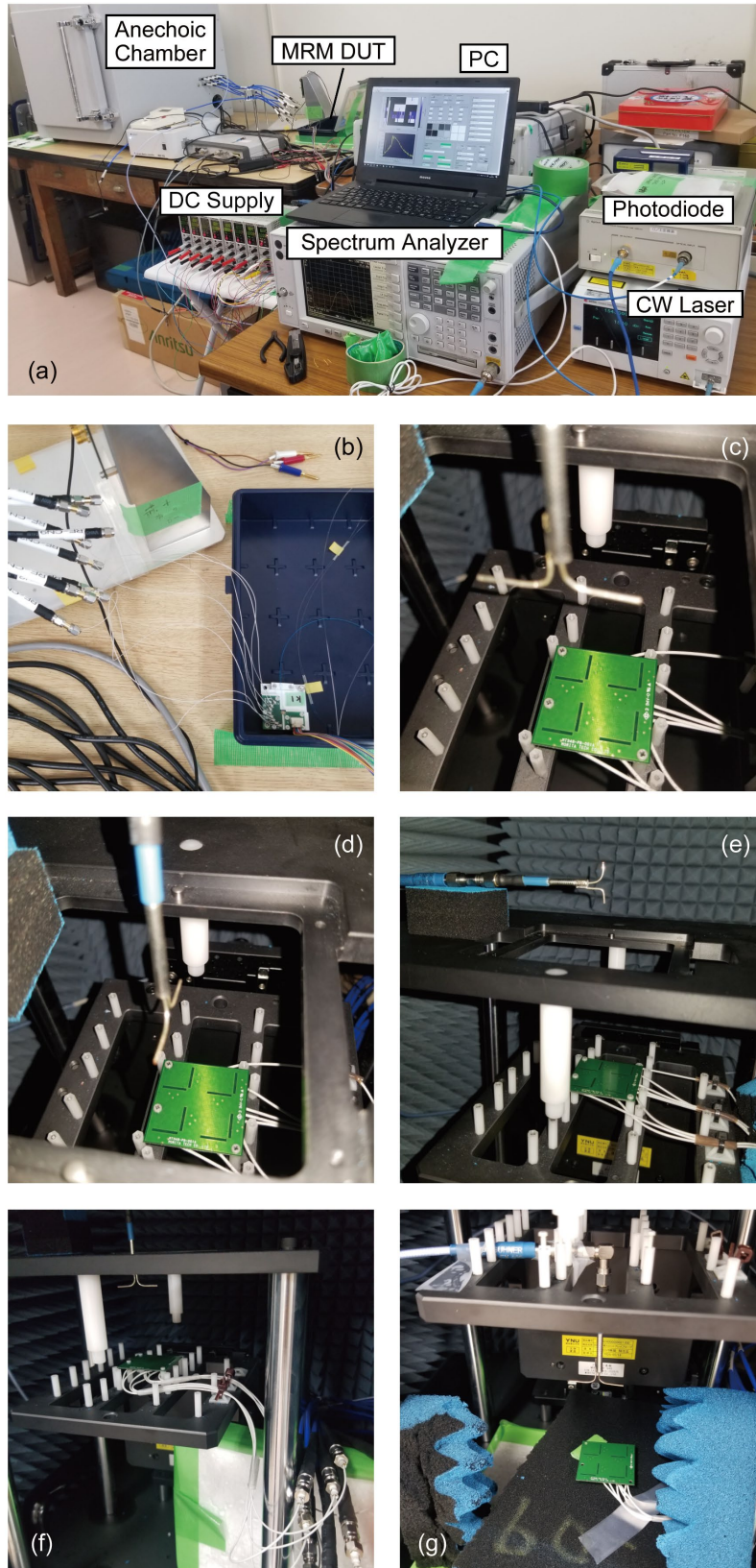
Figure 4-5 Detailed photos of measurement setup. (a) Entail setup. (b) RoF module and its electrical connection with RF probe. (c) x-direction, (d) y-direction and (e) z-direction placement of dipole antenna. Changing the relative position between the dipole antenna and RF probe by moving (f) RF probe and (g) dipole antenna.
