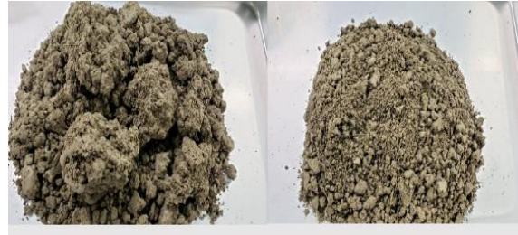
Before crumbling After crumbling
