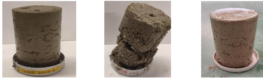
(a) PSAS-N after 5 cycles (b) PSAS-R after 2 cycles (c) BFCB after 5 cycles
