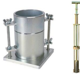
Figure 4.3 Instruments used for Compaction
