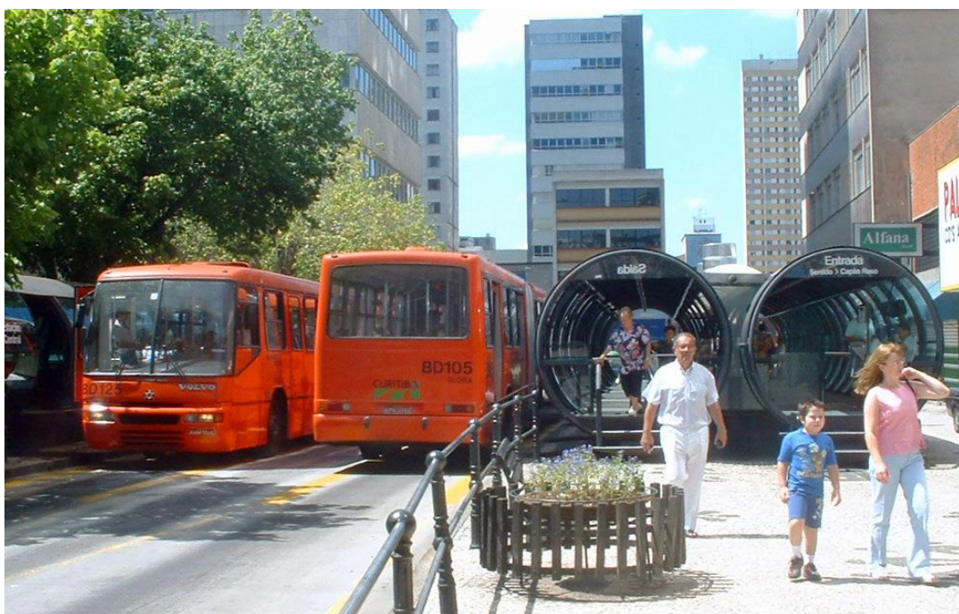
Figure 2.3 Curitiba BRT with buses and tube station. Source: Karl Fjellstrom, Far East Mobility
