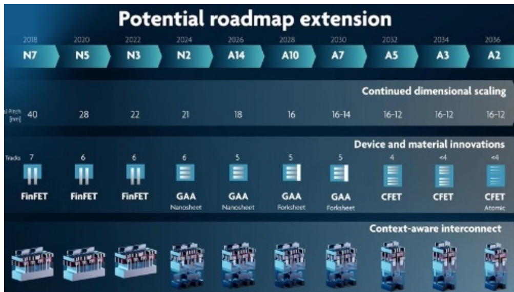
Figure 1.1: Roadmap of miniaturization of CMOS transistor[6]. They said the process rule of state-of-the-art CMOS will reach 0.2 nm in the 2040s.
