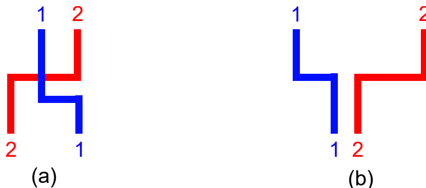
Figure 4.5: (a) has a relationship in the HCG, while (b) does not. In (a), assigning horizontal signal lines to the same track causes overlap, while in (b), this does not occur.
