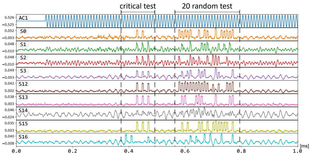
Figure 5.5: Measurement waveform of the 16-bit KSA for 5 critical test vectors shown in Table 5.2 and the first 20 random test vectors shown in Table 5.3. The signals from top to bottom are the excitation current, output bits 0 (LSB) to 3, bits 12-to-15, and the output of the carry (MSB). Critical tests include test cases in which the carry moves from the LSB to the MSB. All tests cases have been validated.
