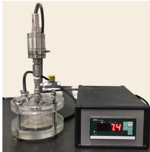
Figure 7.2. Experimental device to evaluate CaCO 3 content
