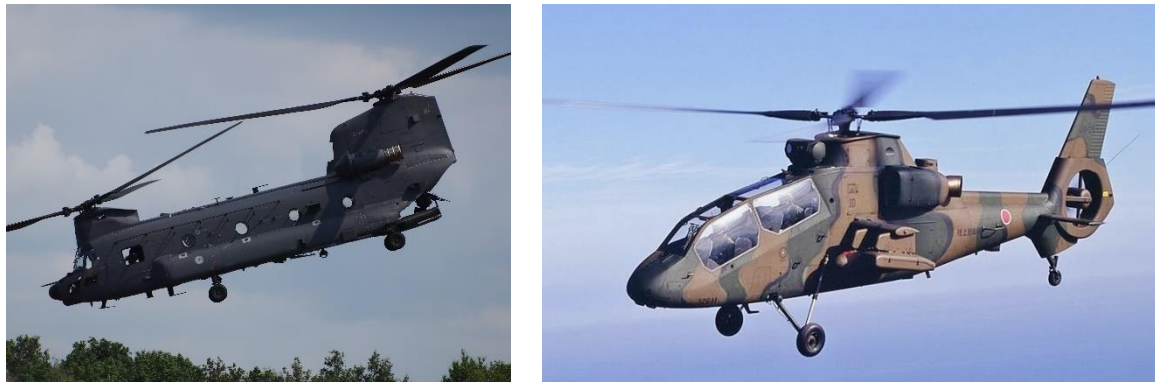
Fig. 4.68 Two kinds of helicopter wing mounting methods
