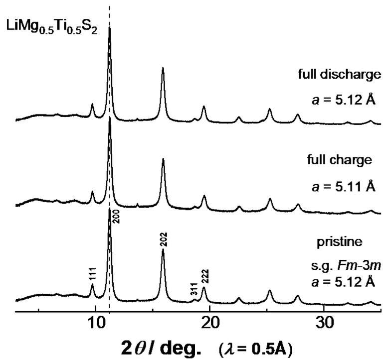
**Figure S6.** Structural changes of rocksalt  $\text{Li}_{1-x}\text{Mg}_{0.5}\text{Ti}_{0.5}\text{S}_2$  measured by *ex-situ* XRD study. Similar to  $\text{Li}_{1-x}\text{Mn}_{0.5}\text{Ti}_{0.5}\text{S}_2$ , a quite small change in the unit cell volume is observed on charge/discharge cycles.
