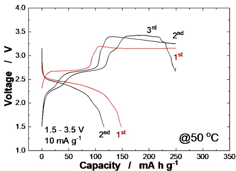
**Figure S4.** Charge/discharge curves of layered  $\text{LiMn}_{0.5}\text{Ti}_{0.5}\text{S}_2$  at  $50\text{ }^\circ\text{C}$  at a rate of  $10\text{ mA g}^{-1}$ .
