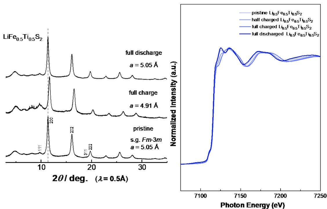
**Figure S5.** Structural changes of rocksalt  $\text{Li}_{1-x}\text{Fe}_{0.5}\text{Ti}_{0.5}\text{S}_2$  measured by *ex-situ* XRD study. Changes in Fe K-edge
