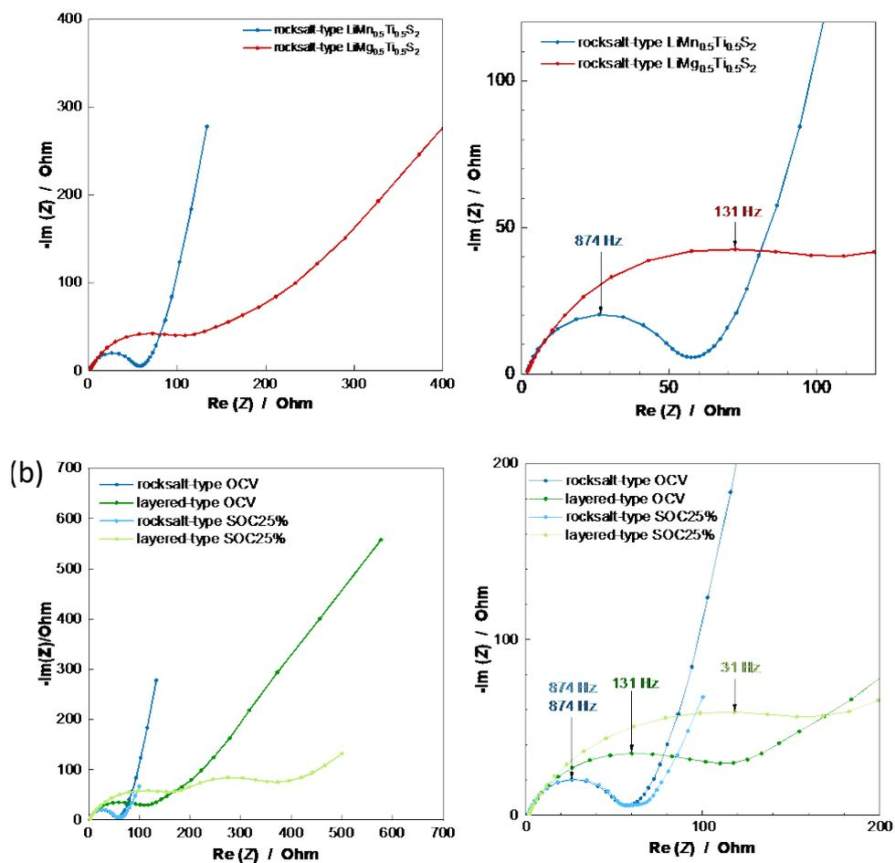
**Figure S3.** (a) Comparison of impedance measured at an open-circuit voltage (OCV) condition without electrochemical cycle for  $\text{LiMn}_{0.5}\text{Ti}_{0.5}\text{S}_2$  and  $\text{LiMg}_{0.5}\text{Ti}_{0.5}\text{S}_2$  with the rocksalt structure, and (b) impedance of rocksalt and layered  $\text{LiMn}_{0.5}\text{Ti}_{0.5}\text{S}_2$  measured at OCV and 25% state of charge (SOC).
