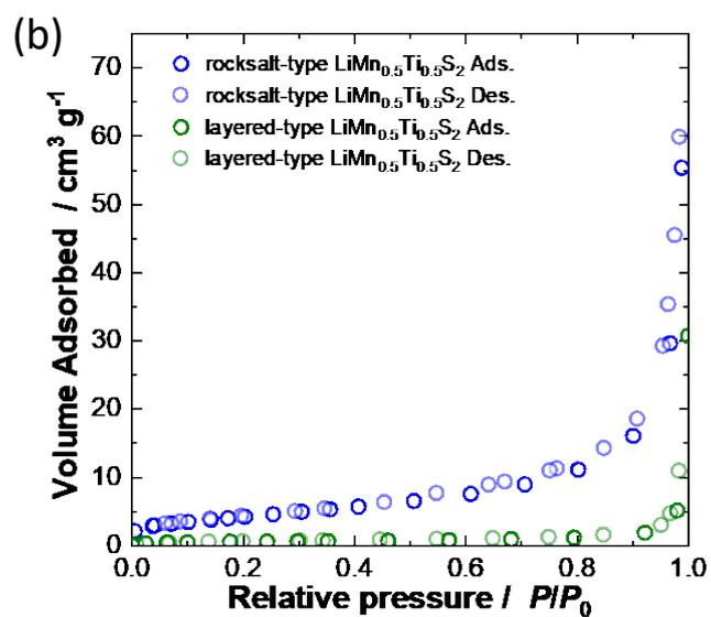
**Figure S1.** (a) SEM images of cation-disordered rocksalt and cation-ordered layered  $\text{LiMe}_{0.5}\text{Ti}_{0.5}\text{S}_2$  ( $Me = \text{Fe}^{2+}$ ,  $\text{Mn}^{2+}$ , and  $\text{Mg}^{2+}$ ). (b) Results of BET specific surface area measurement for rocksalt and layered  $\text{Li}_{1-x}\text{Mn}_{0.5}\text{Ti}_{0.5}\text{S}_2$  samples.
