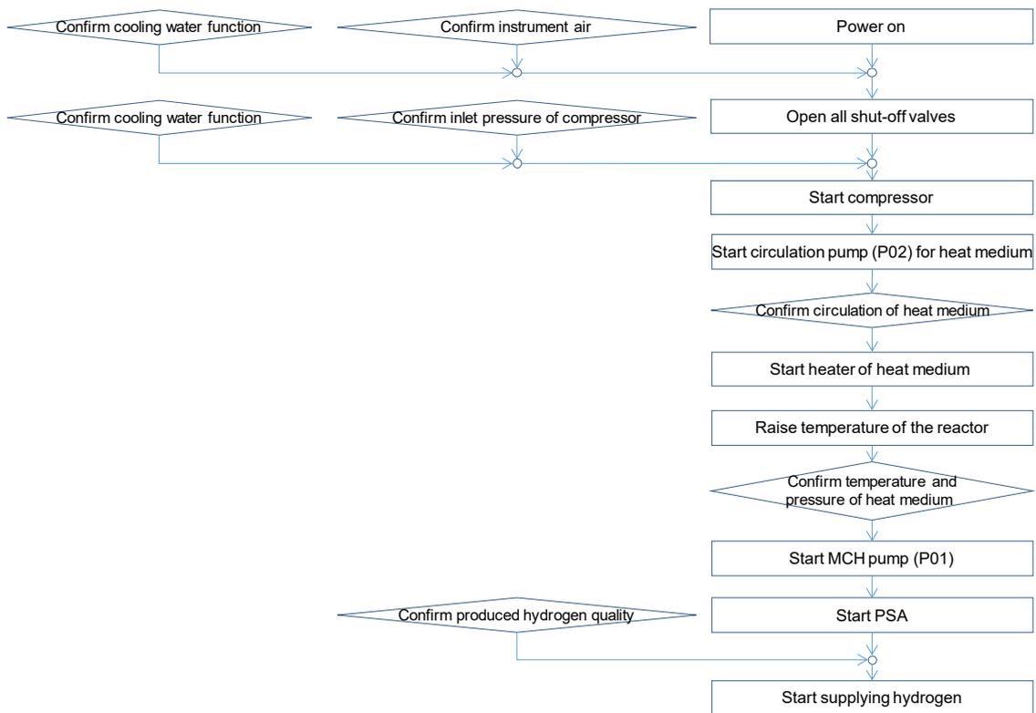
Fig. 4. Startup operational procedure of the dehydrogenation process.
