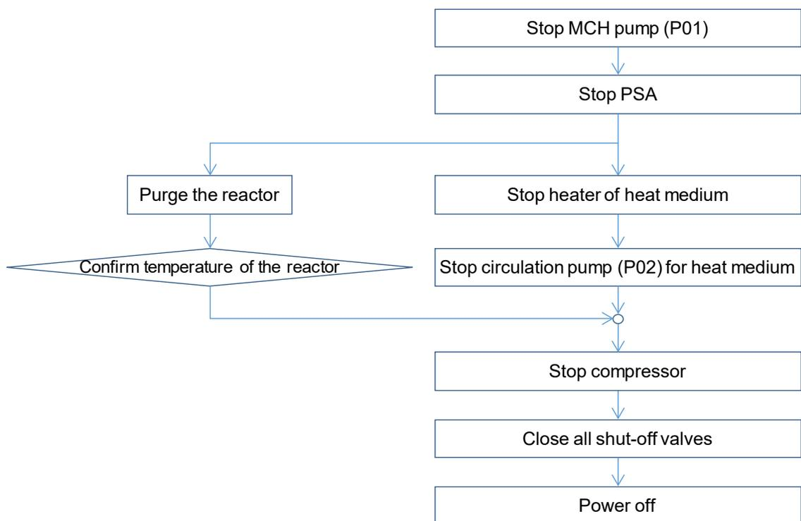
Fig. 5. Shutdown operational procedure of the dehydrogenation process.
