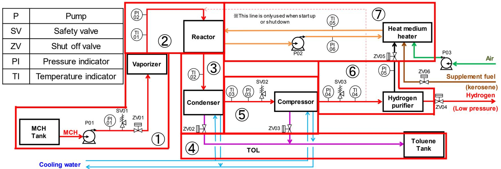
Fig. 1 Simple flow of the dehydrogenation process.
