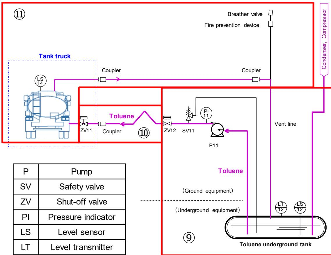
Fig. 3. Simple flow of the loading toluene process.
