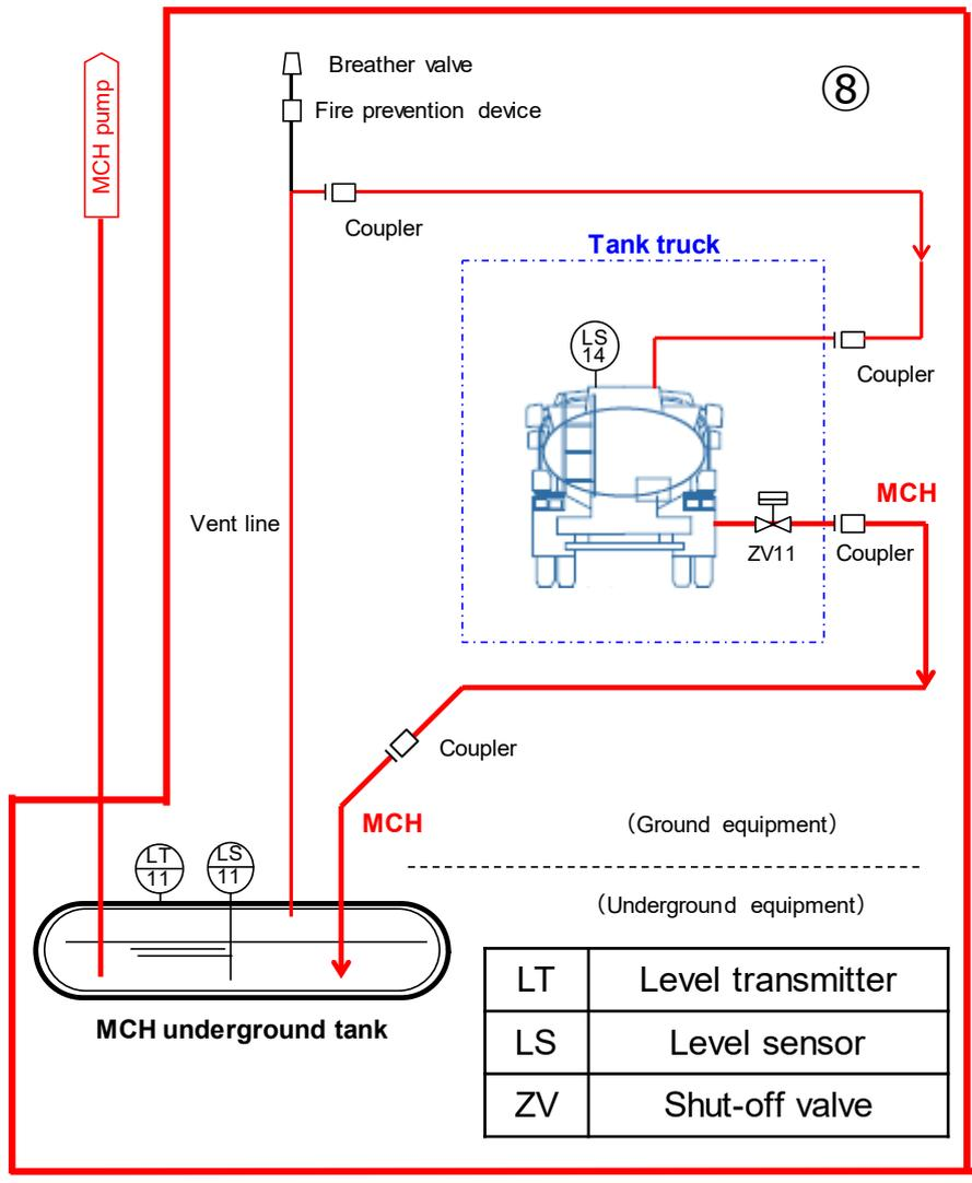
Fig. 2. Simple flow of the unloading MCH process.
