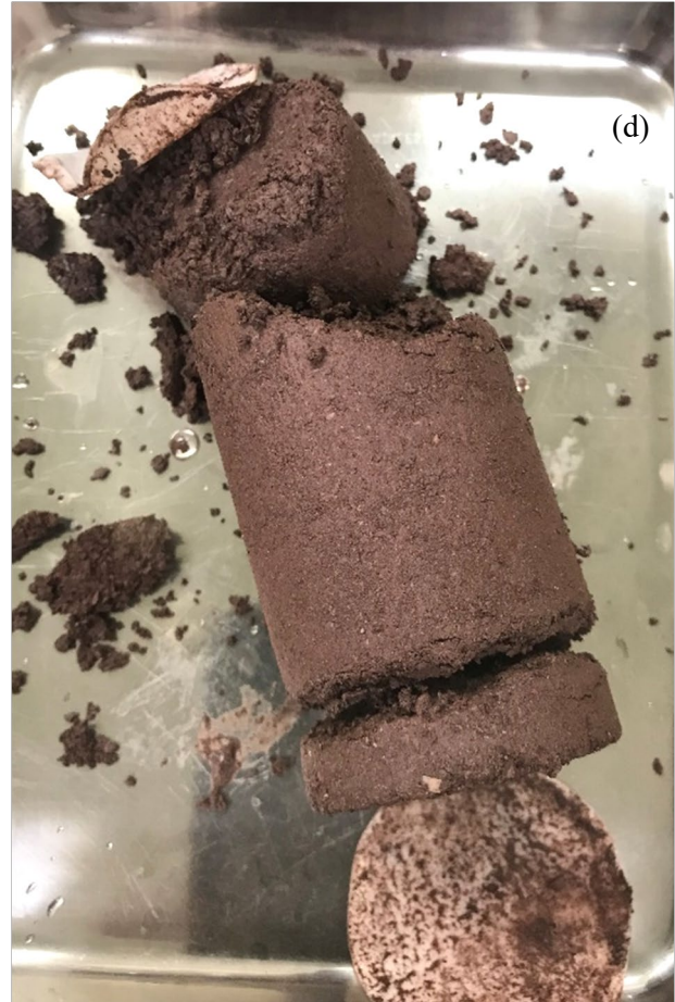
Fig. 8 (a) Soil sample before testing, (b) soil specimen after consolidation, (c) bulging failure of soil specimen after shearing, and (d) soil specimen after testing
