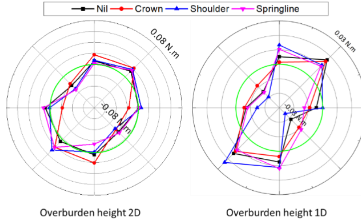
Figure 4-36. Effect of weak zone position on bending moment at maximum shear displacement
