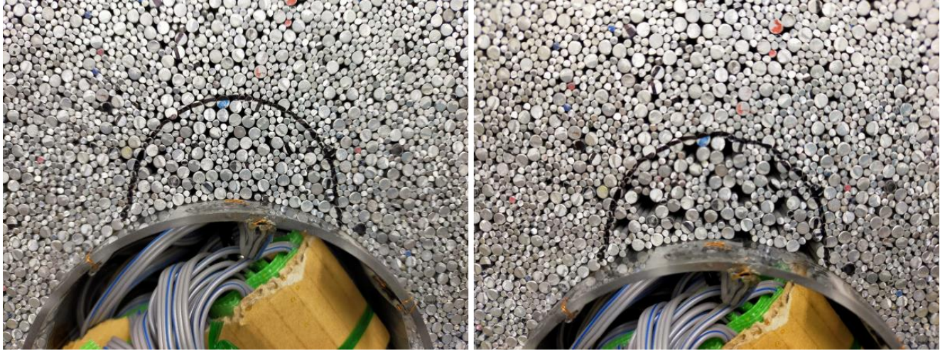
Figure 3-15. Ground condition before and after the creation of the weak zone
