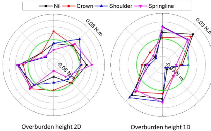
Figure 4-35. Effect of weak zone position on bending moment at the completion of 30 th cycle ( e = 0.45 )
