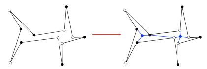
Figure 3: Non-quadrangulatable polygon P and a quadrangulation of P with two Steiner points
