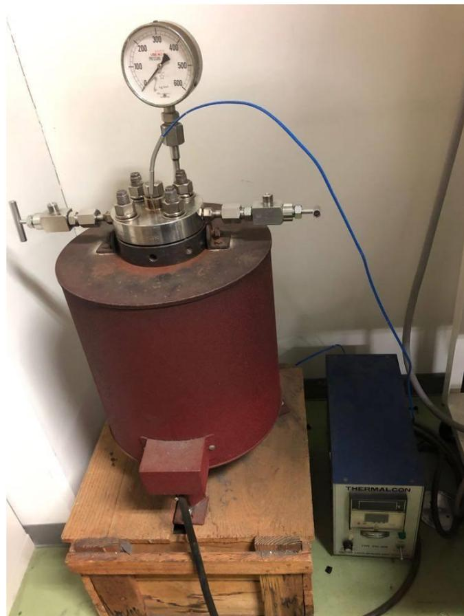
**Fig. 2-2** Photo for the used autoclave, Yokohama National University.
