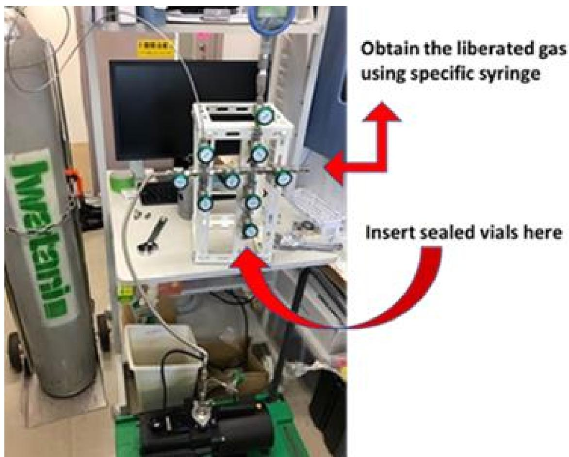
**Fig. 4-2** Gas Extraction System in JAMSTEC
