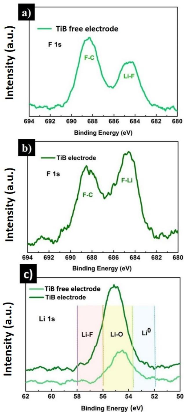
**Fig. S13** XPS spectra of Li anode surfaces after 30 charge/discharge cycles (**Fig. S10b**) of the TiB-free and TiB electrode pouch cells with the [Li(SL)<sub>2</sub>][TFSA]-4HFE electrolyte: a), b) F 1s spectra of the TiB free and TiB electrode, respectively, and c) Li 1s spectra.
