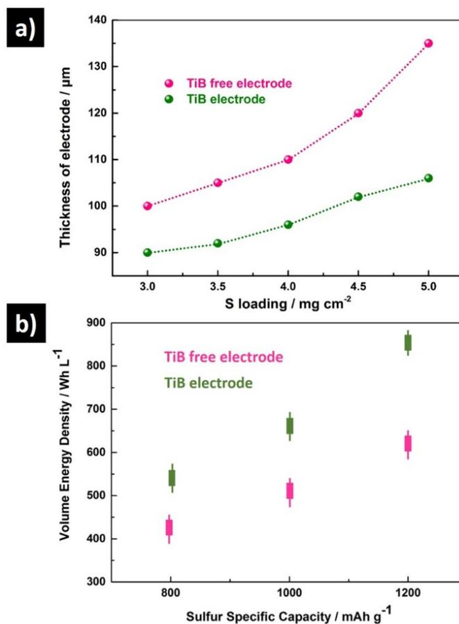
**Fig. S9** a) Thickness of the TiB free and TiB electrodes under different S loadings, b) Volume energy density range of Li-S battery with the corresponding electrode thickness under S loading of  $5 \text{ mg cm}^{-2}$ . The calculation is based on  $2 \text{ Ah}$  pouch cell.
