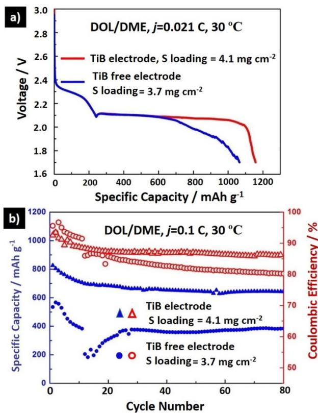
**Fig. S5** a) Initial discharge curves of the TiB and TiB free electrodes at 0.021 C and b) subsequent cycling performance and Coulombic efficiency at 0.1 C with 1 M Li[TFSA] in DOL/DME containing 0.5 wt% LiNO<sub>3</sub> at E/S = 10  $\mu\text{L mg}^{-1}$ .
