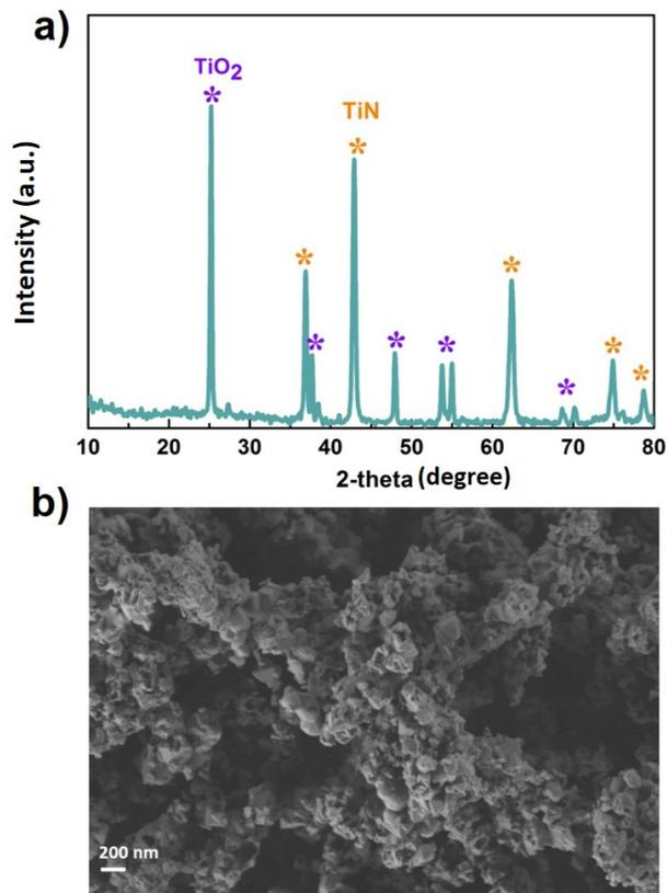
**Fig. S2** a) XRD pattern and b) SEM image of the TiB material. The peaks at 36.9°, 43.1°, 62.5°, 74.9°, and 78.7° can be assigned to the (111), (200), (220), (311), and (222) reflections of crystalline TiN, respectively.<sup>7</sup> The other peaks at 25.3°, 37.7°, 48.0°, 55.0°, and 70.0° are ascribed to the reflections from the (101), (004), (200), (105), and (211) planes of TiO<sub>2</sub>, respectively.<sup>8</sup>
