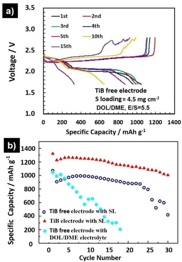
**Fig. S12** a) Discharge curves of a pouch cell at 0.1 C using the TiB free electrode and DOL/DME electrolyte at an E/S ratio of 5.5. b) Cycling performance of pouch cells at 0.1 C using the TiB free and TiB electrodes at an E/S ratio of 5.5. The electrolytes were either DOL/DME or [Li(SL)<sub>2</sub>][TFSA]-4HFE.
