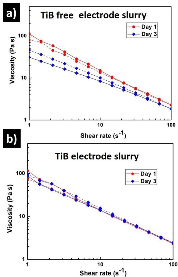
**Fig. S4** Variation in viscosity with shear rate of the a) TiB free electrode slurry and b) TiB electrode slurry on the first day (Day 1) and third day (Day 3) after preparation TiB free. Solid and broken lines correspond to measurements taken with increasing and decreasing shear rate, respectively.
