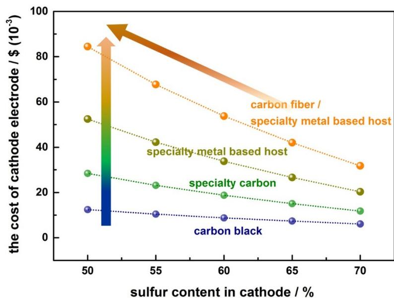
**Fig. S1** Cost of sulfur cathode based on a 2 Ah pouch cell with various kinds of carbon material. The lowest cost cathode is based on carbon black, and the highest is with the carbon fiber materials.<sup>6</sup>
