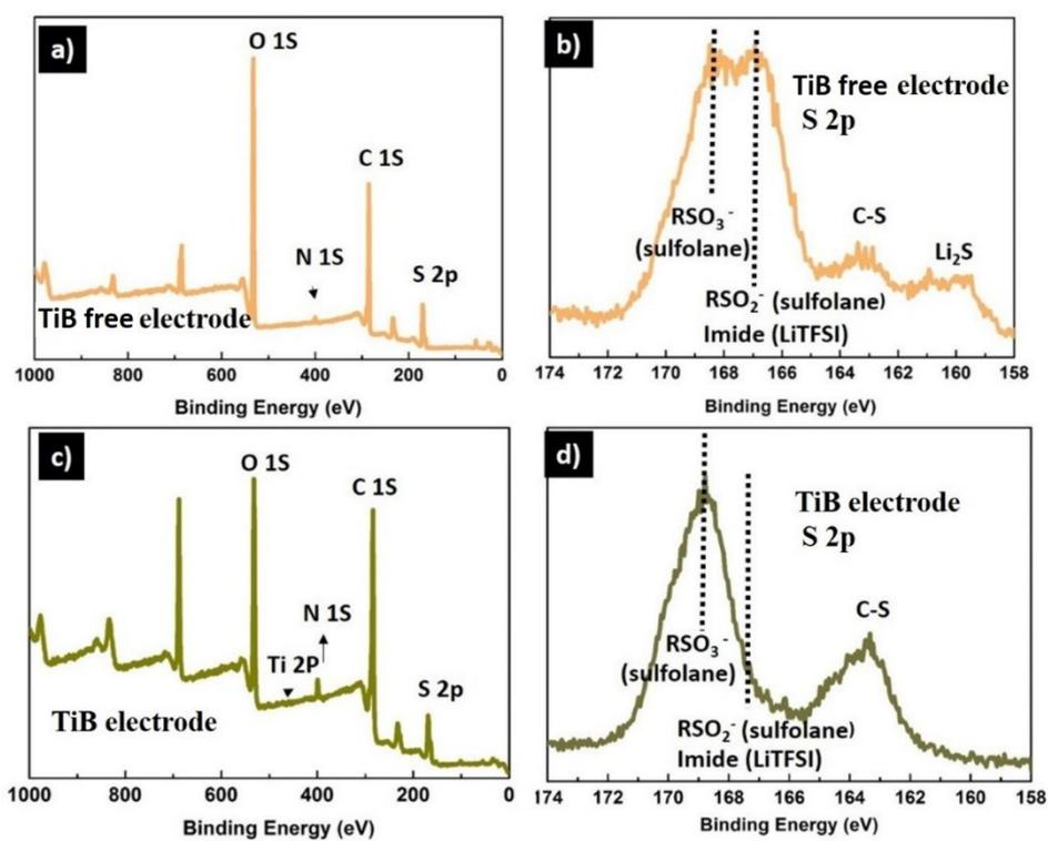
**Fig. S7** XPS spectra of the electrodes in the charged state after 200 cycles at 0.1 C (after the experiments shown in **Fig. 5b**): a) and c) XP survey spectra of the TiB free and TiB electrode, respectively and c) and d) high-resolution S 2p XP spectra of the TiB free and TiB electrode, respectively.
