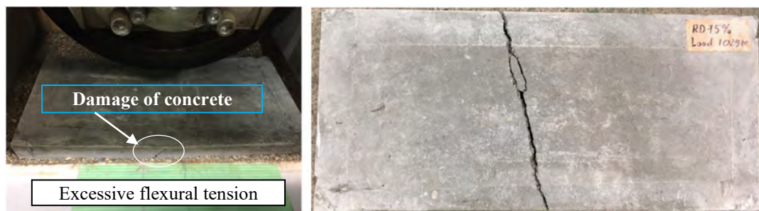
Fig. 3-21 The failure mode of concrete slab 20mm with the static load 1,029N and RD 75%.
