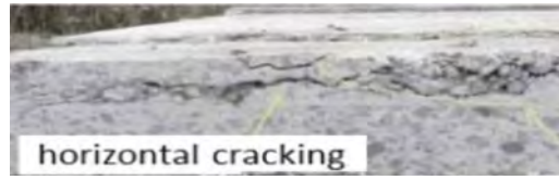
Fig. 7-8 Horizontal cracking at top surface of concrete bridge deck under moving loads [16].
