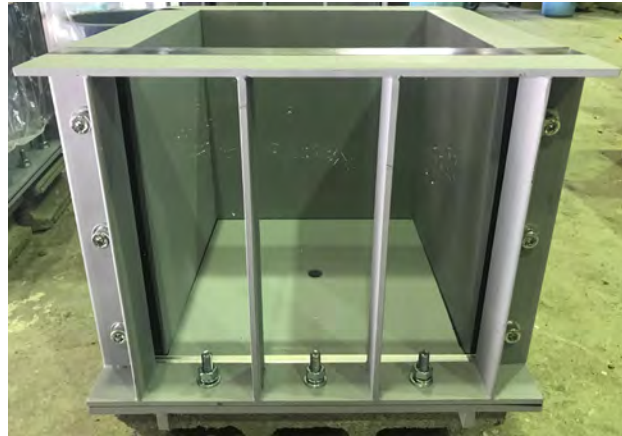
Fig. 3-2 Sand formwork for experiment.
