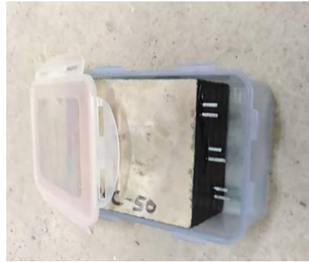
Type B: Vinyl Electric Insulation Tape with Polypropylene Lidded Container
