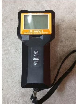
Figure 4-4 Kett HI-520-2 surface moisture meter
