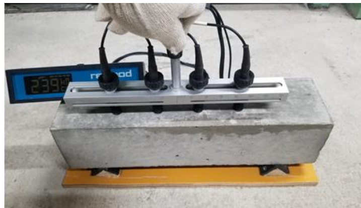
Figure 4-6 Surface electrical resistivity measurement
