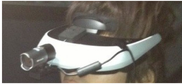
Figure 1. Apparatus (HMD and Camera) used in the food appearance modification experiments reported here.
