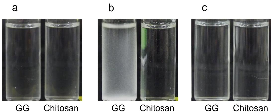
Fig. S4. Reversible insolubilization of GG in response to temperature. GG or chitosan (5 mg) was dissolved in 5 mL of 10 mM HCl containing 1 M NaCl. The solutions were kept at 25 °C for 24 h (a) and then at 4 °C for 24 h (b). After cooling, the solutions were heated at 50 °C for 2 min (c). Chitosan used for the experiment has deacetylation degree of 90% and molecular weight of  $\geq 1 \times 10^5$  Da.
