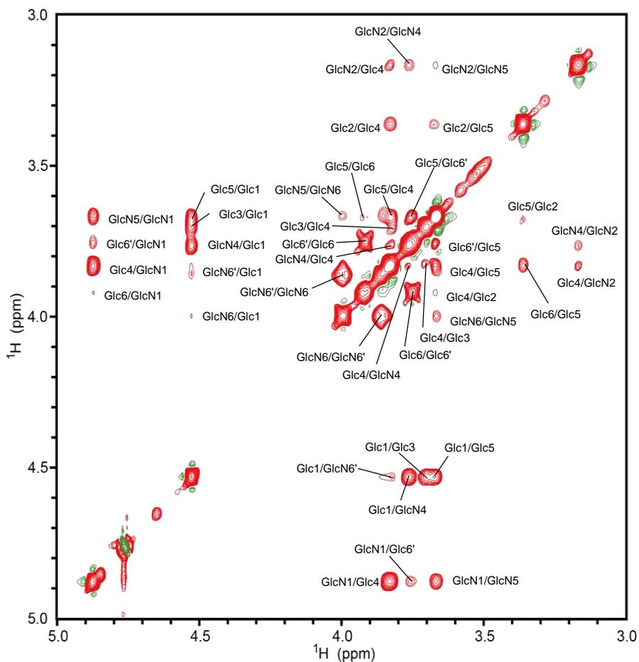
Figure S2. NOESY spectrum (80 ms) of GG. The crosspeaks (NOE signals) identified are designated as GlcN1/Glc4 (correlation between H1 of GalN and H4 of GlcN), etc. Positive and negative signals are indicated in red and green lines, respectively.
