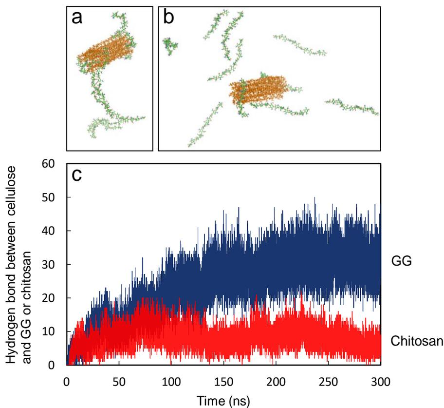
Figure S5. Adsorption of GG onto cellulose during MD simulation. The snapshots of the GG-cellulose (a) and chitosan-cellulose (b) systems at 300 ns show that cellulose adsorbs GG much more than chitosan. This observation was supported by the time courses of the number of hydrogen bond between cellulose and GG or chitosan during the simulations (c).
