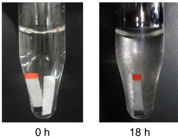
Figure S6. Cellulase tolerance of GG-treated cellulose. GG-treated (indicated by red and black edges) and non-treated paper strips were soaked in cellulase solution followed by incubation at 45 °C for 18 h.
