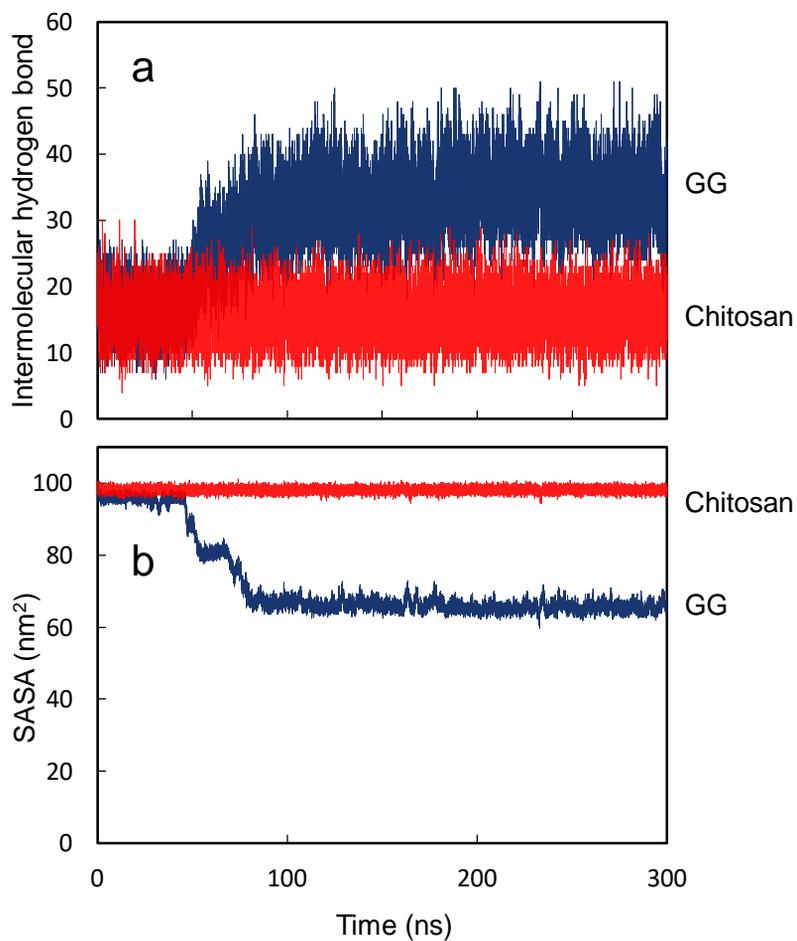
Figure S3. Time courses of interchain hydrogen bond number (a) and the total solvent-accessible surface area (b) during MD simulation of GG or chitosan chain (12 mer) in water. The data for GG correspond to the simulation whose structure is shown in Fig. 2. Abbreviation: SASA, total solvent-accessible surface area.
