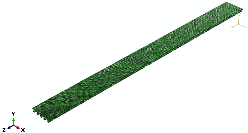
Fig 5.11 ABAQUS model of the viaduct
