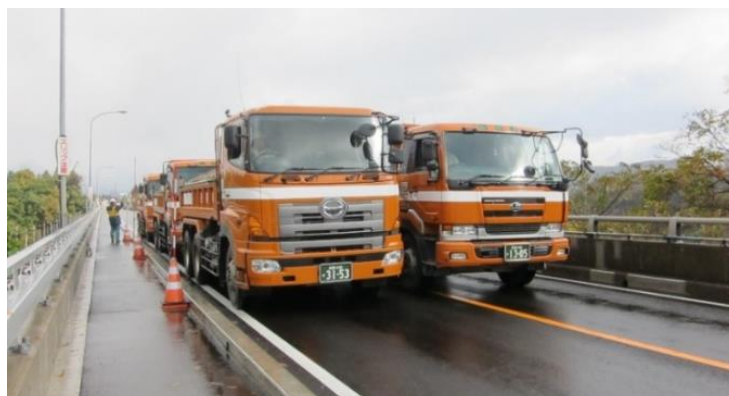
Fig 2.2 Static proof load test on Myoko Bridge in Nov, 2011
