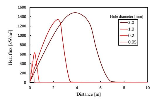
Fig. 6: Heat flux as a function of distance
