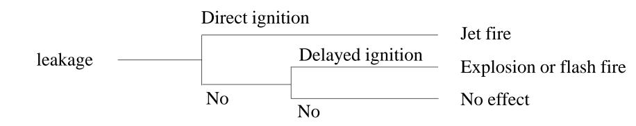
Fig. 3: Hydrogen leakage event tree
