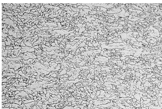
(b) Bainitic ferrite steel, DBTT = -100 °C
