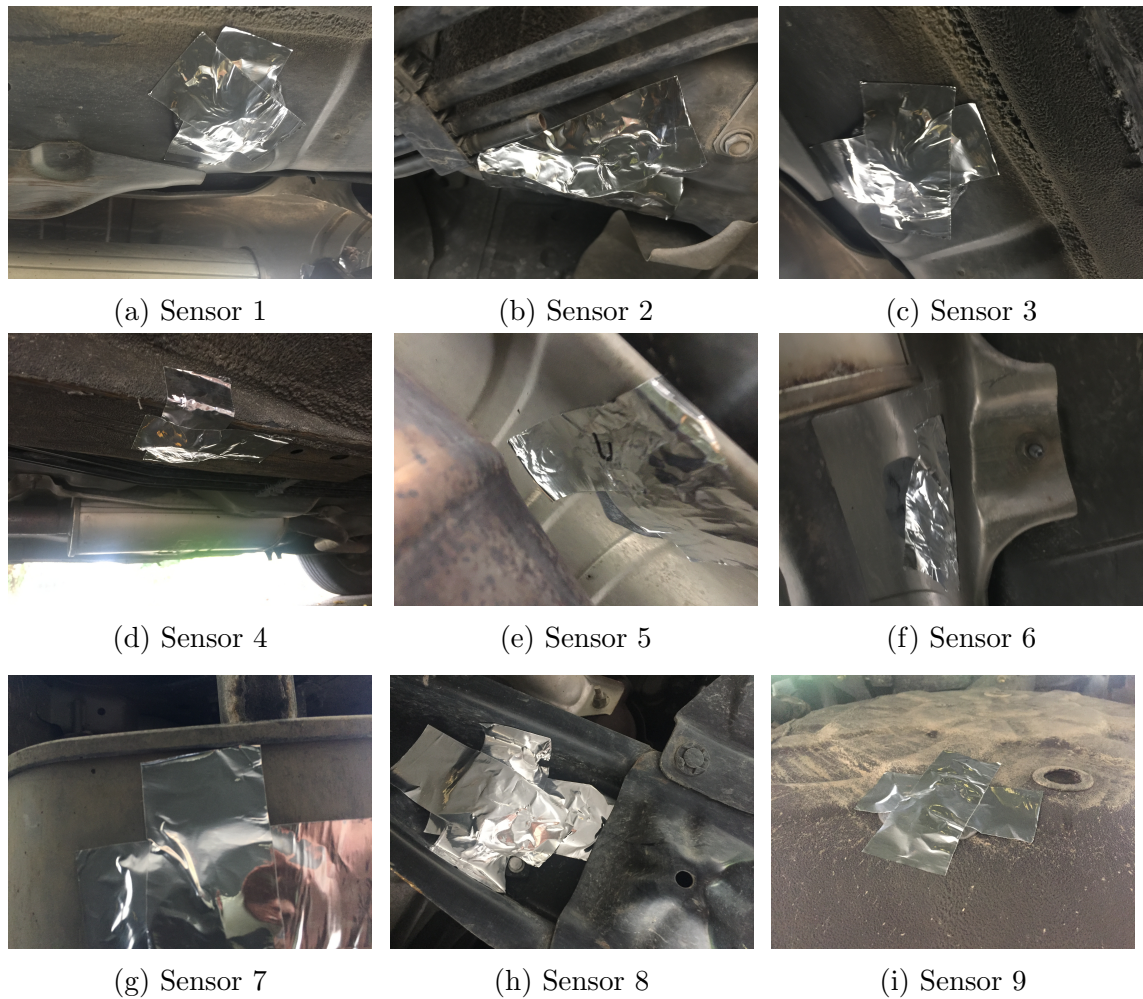
Figure 3.9: Sensors attachment at car bottom
