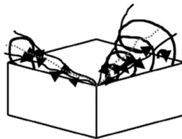
Figure 2-5: Strong conical vortex to induce high peak suction (Kawai 2002)
