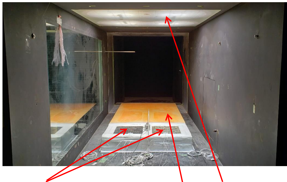
Asphalt specimen, Panel to prevent the turbulency, Heat-Lamps
