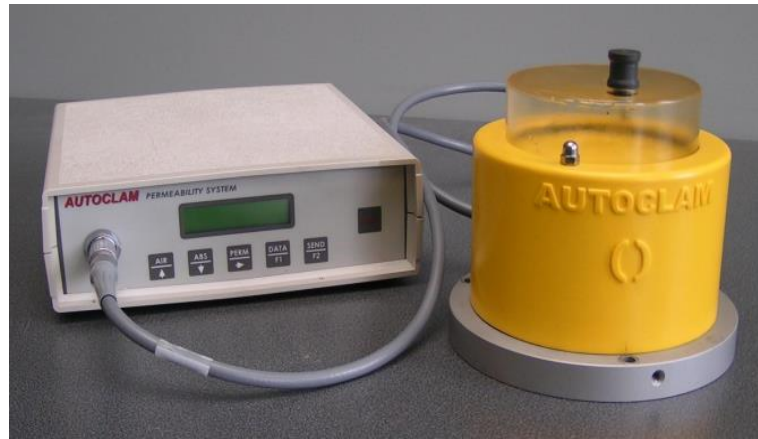
Fig.2.7 Schematic diagram of Autoclam air permeability test [2.12]
