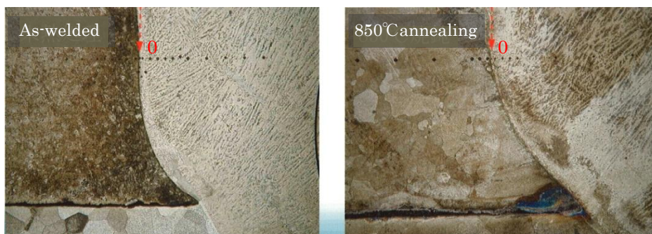
Fig. 5.4 Marks of Vickers hardness test in MIG S1/W2/S4 joint. 0 is the weld interface
