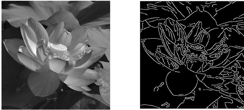
(a) Original image (b) Edges found using Canny-Edge-Detection
