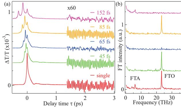
**Fig. 2.** (a) Transient transmission change of 4H-SiC. The red curve shows the result excited by single pulses, while others are the results excited by pulse trains consists of three pulses with different pulse intervals  $\Delta t = 45$  fs, 65 fs, 85 fs, and 152 fs. After  $\tau = 1$  ps, all data were magnified by 60 for clarity. (b) Fourier transformed power spectra of (a) carried out 1 ps to 5 ps.
