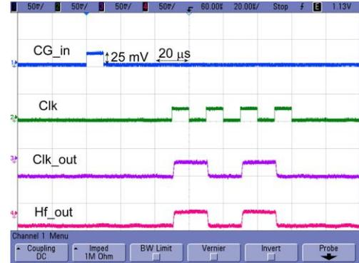
Fig. 6. High-speed measurement result of the four-input merger using a SQUID stack. Because the SFQ output is detected by the SFQ/dc converter, the transition of the voltage level of the Out signal corresponds to the output of the SFQ signal.
