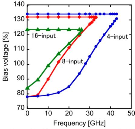
Fig. 4. Dependence of the bias voltage margin of the multi-input mergers using a SQUID stack on their operating frequency. The bias voltage is normalized at 2.5 mV.
