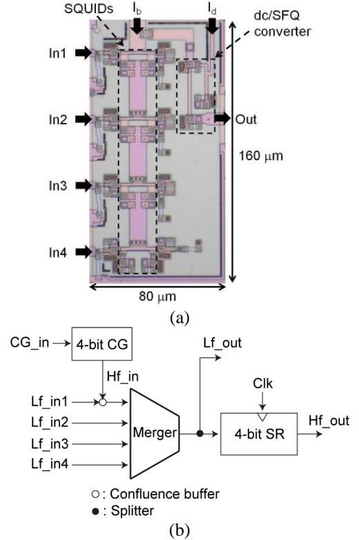
Fig. 5. (a) Microphotograph of the four-input merger using a SQUID stack and (b) block diagram of the test circuit of the four-input merger.
