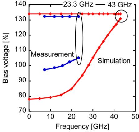
Fig. 7. Comparison of the measured and simulated results of the dependence of the bias voltage of the four-input merger using a SQUID stack on its operating frequency. In this measurement,  $I_{\text{offset}}$  of 380  $\mu\text{A}$  was supplied.
