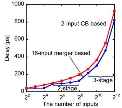
Fig. 8. Dependence of the delay on the number of inputs of the merging circuit.
