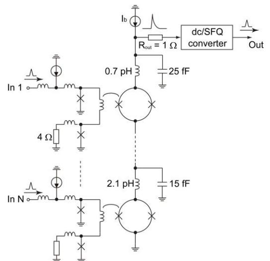
Fig. 1. Circuit schematic of an  $N$ -input merger using a SQUID stack. The critical current of JJs composing the dc-SQUID stack is  $200 \mu\text{A}$ . The loop inductance of each dc-SQUID is  $5.02 \text{ pH}$ . The mutual inductance between the JTL and dc-SQUID loop is  $2.24 \text{ pH}$ .
