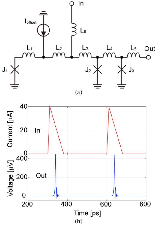
Fig. 2. (a) Equivalent circuit of the dc/SFQ converter used in the designed multi-input merger and (b) its simulation result.  $J_1 = 184 \mu\text{A}$ ,  $J_2 = 163 \mu\text{A}$ ,  $J_3 = 199 \mu\text{A}$ ,  $L_1 = 4.83 \text{ pH}$ ,  $L_2 = 2.80 \text{ pH}$ ,  $L_3 = 0.03 \text{ pH}$ ,  $L_4 = 9.41 \text{ pH}$ ,  $L_5 = 5.11 \text{ pH}$ ,  $L_6 = 3.42 \text{ pH}$ , and  $I_{\text{offset}} = 350 \mu\text{A}$ .
