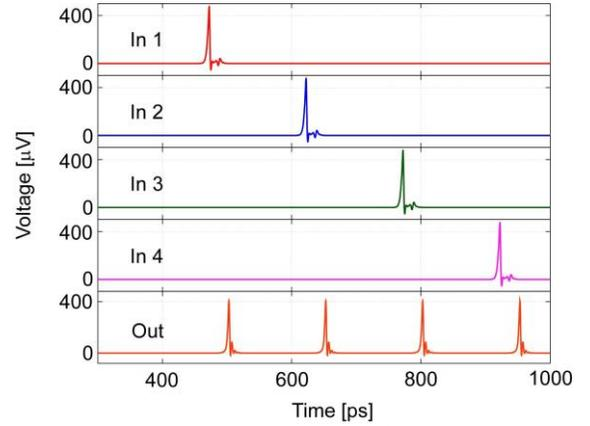
Fig. 3. Simulated input and output waveforms of a four-input merger using a SQUID stack.
