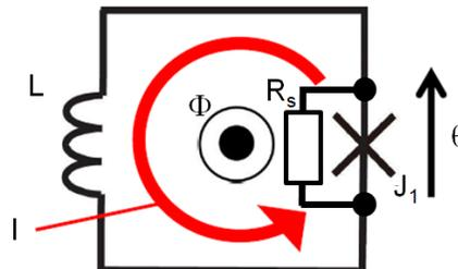
Fig.1. Equivalent circuit of an rf-SQUID. L is inductance consisting rf-SQUID loop. J<sub>1</sub> is Josephson junction.  $\Phi$  is internal magnetic flux in rf-SQUID, I is the circular current. R<sub>s</sub> is shunt resistance of Josephson junction J<sub>1</sub>.  $\theta$  is the phase difference of the macroscopic wave function across the Josephson junction J<sub>1</sub>.
