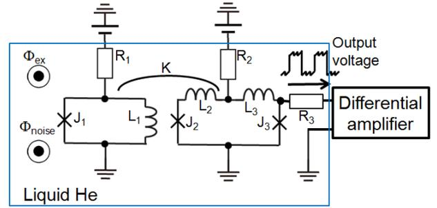
Fig. 5. Circuit schematic of the measured rf-SQUID memory cell. The dc-SQUID detects datum write/read. The external magnetic flux  $\Phi_{ex}$  and the noise magnetic flux  $\Phi_{noise}$  are applied to the rf-SQUID from a room-temperature instrument.  $J_1 = 50 \mu\text{A}$ ,  $J_2 = J_3 = 100 \mu\text{A}$ ,  $L_1 = 30.3 \text{ pH}$ ,  $L_2 = L_3 = 3.5 \text{ pH}$ ,  $R_1 = R_2 = 500 \Omega$ ,  $R_3 = 7.5 \Omega$ ,  $k = 0.3$  is magnetic coupling coefficient between  $L_1$  and  $L_2, L_3$ .
