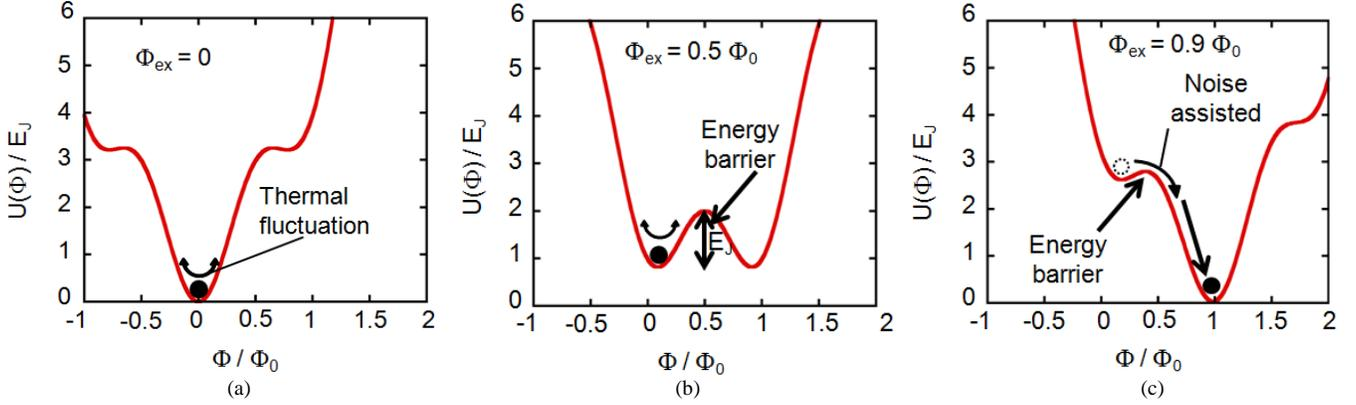
Fig. 2. Potential energy diagrams of rf-SQUID. (a)  $\Phi_{ex} = 0$ , (b)  $\Phi_{ex} = 0.5 \Phi_0$ , (c)  $\Phi_{ex} = 0.9 \Phi_0$ .  $\Phi_{ex}$  is the external magnetic flux uniformly applying to whole of the rf-SQUID,  $\Phi_0 = 2.07 \times 10^{-15}$  Wb is single flux quantum,  $E_J$  is Josephson energy.  $L = 30.1$  pH,  $J_I = 50$   $\mu$ A in Fig. 1.  $E_J = 1.68 \times 10^{-20}$  J, corresponds to 1200 K thermal energy.
