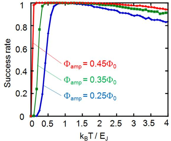
Fig. 3. Simulated dependences of the success rate of the read/write operation of the rf-SQUID memory cell on the noise energy when  $\Phi_{amp}$  is  $0.25\Phi_0$ ,  $0.35\Phi_0$  and  $0.45\Phi_0$ . The horizontal axis is normalized by Josephson energy  $E_J$ .  $k_B$  is the Boltzmann constant.
