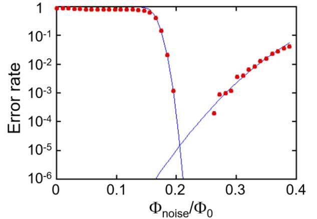
Fig. 7. Dependence of the measured error rate of the read/write operation of the 1-bit rf-SQUID memory cell on the amplitude of the standard deviation of magnetic flux noise  $\Phi_{noise}$ . Dots are measurement results. Solid curves are fitting characteristics.
