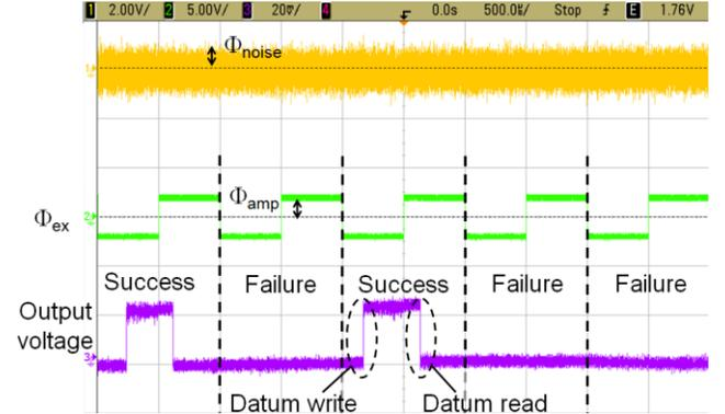
Fig. 6. Measured waveform of write/read operation of the rf-SQUID memory cell. The dc-SQUID is properly biased to detect datum write/read.  $\Phi_{ex}$  is the inverse of the current supplied to the memory cell.  $\Phi_{amp}/\Phi_0$  was 0.25 in this measurement. Because the noise condition was not optimum, long delay of datum write was observed.
