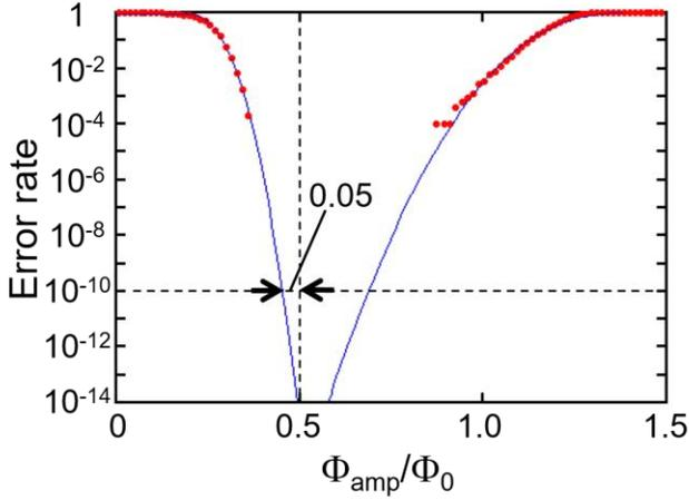
Fig. 4. Simulated dependences of the error rate of the read/write operation of the rf-SQUID memory cell on the input magnetic flux amplitude  $\Phi_{amp}$  when  $k_B T/E_J$  is 0.42. The horizontal axis is normalized by single flux  $\Phi_0$ .  $k_B$  is the Boltzmann constant. Solid curves are fitting characteristics based on the error function.
