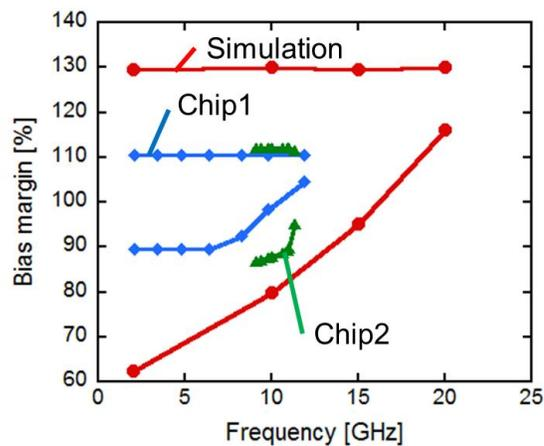
Fig. 10. Dependence of the bias margin of the operating frequency of 8-bit SR using proposed technique. The bias margin is normalized by the designed bias voltage, 0.25 mV.
