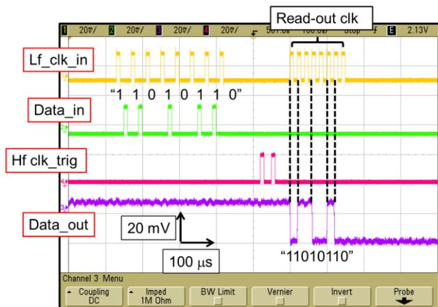
Fig. 9. Measurement waveform of 8-bit SR using proposed technique. The “Hf\_clk\_trig” is trigger signal for the 8-bit clock generator.
