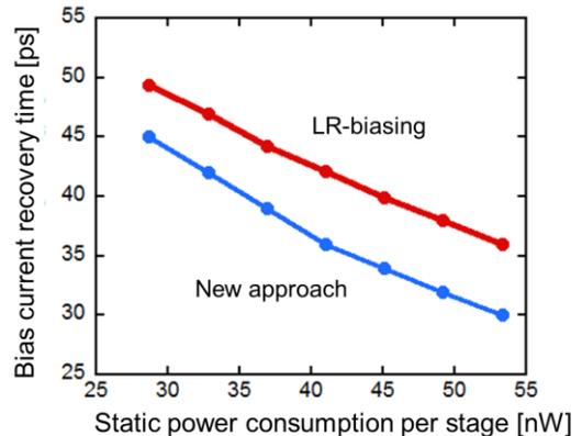
Fig. 3. Dependence of the bias current recovery time of conventional and new LR-biased JTLs on static power consumption per stage.
