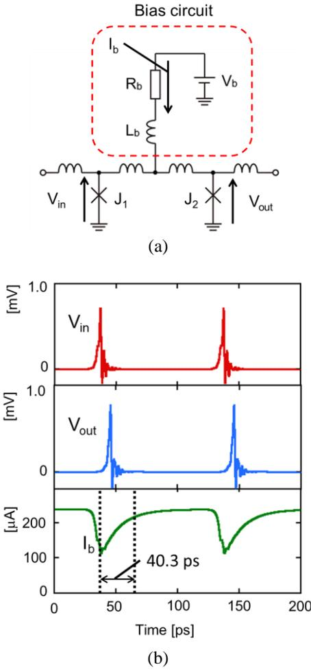
Fig. 1. (a) Equivalent circuit of a 1-stage LR-biased Josephson transmission line (JTL) and (b) its simulation result.  $J_1 = J_2 = 216 \mu\text{A}$ ,  $L_b = 10 \text{ pH}$ ,  $R_b = 0.84 \Omega$ ,  $V_b = 0.2 \text{ mV}$ .
