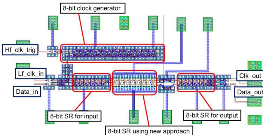
Fig. 8. Layout of the test circuit of the 8-bit SR using proposed technique and whole measurement circuits.
