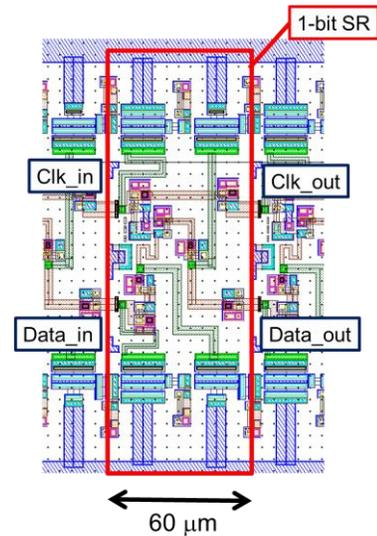
Fig. 7. Layout of 1-bit shift register using the proposed biasing scheme.
