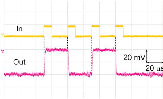
Fig. 5. Measured waveform of 10-stage JTL using the proposed biasing scheme.
