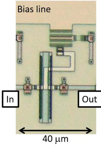
Fig. 4. Microphotograph of the 1-stage JTL with the proposed biasing scheme.
