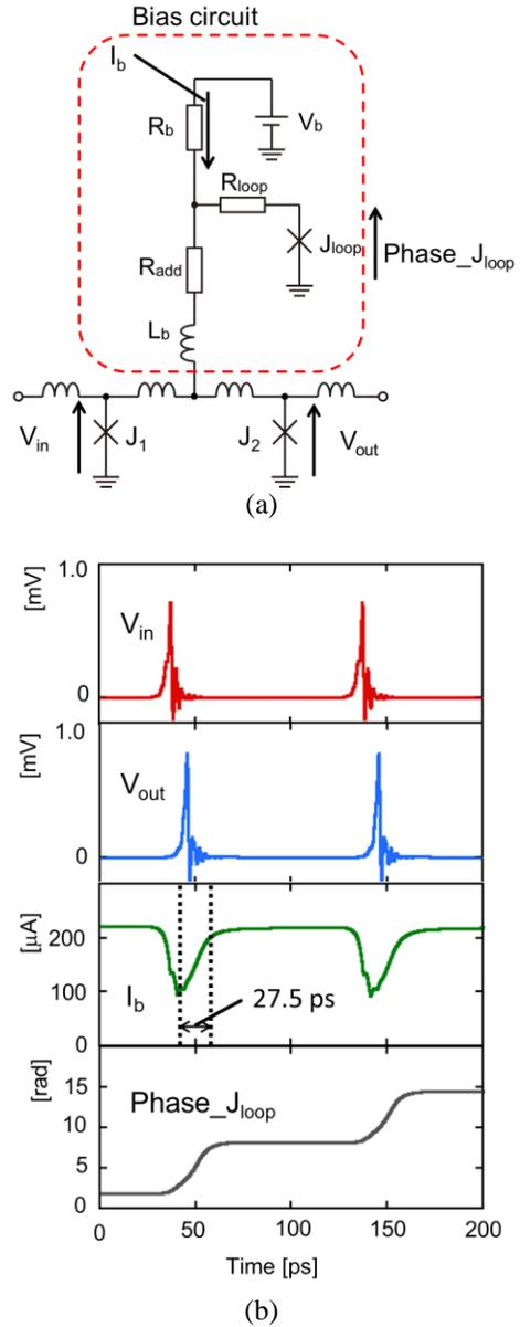
Fig. 2. (a) Equivalent circuit of a 1-stage LR-biased JTL with a dynamic resetting mechanism and (b) its simulation result.  $J_1 = J_2 = 216 \mu\text{A}$ ,  $L_b = 10 \text{ pH}$ ,  $R_b = 0.84 \Omega$ ,  $R_{loop} = 0.4 \Omega$ ,  $R_{add} = 0.05 \Omega$ ,  $J_{loop} = 45 \mu\text{A}$ ,  $V_b = 0.2 \text{ mV}$ .
