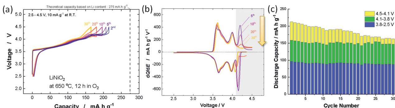
Fig. 1 (a) Galvanostatic charge/discharge curves of  $\text{LiNiO}_2$  at a rate of  $10\text{ mA g}^{-1}$ , (b) differential  $dQ/dE$  plots obtained from (a), and (c) variations in discharge capacities with different voltage ranges.
