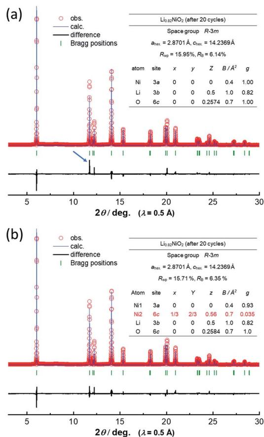
Fig. 4 Comparison of fitting results of Rietveld analysis of the synchrotron XRD pattern of Li<sub>x</sub>NiO<sub>2</sub> after the 20-cycle test (a) without and (b) with the presence of Ni ions at 6c tetrahedral sites. A clear deviation between simulated and observed patterns for the 101 diffraction line is noted in (a) as marked by the blue arrow.
