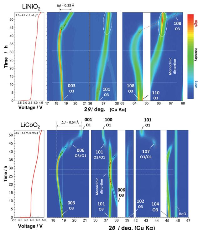
Fig. 2 Contour plots for selected ranges obtained from the *in situ* XRD patterns of  $\text{LiNiO}_2$  and  $\text{LiCoO}_2$  at a rate of  $5 \text{ mA g}^{-1}$ , and corresponding initial charge curves in electrochemical cells are also shown. The original *in situ* XRD data are shown in ESI Fig. S3.†
