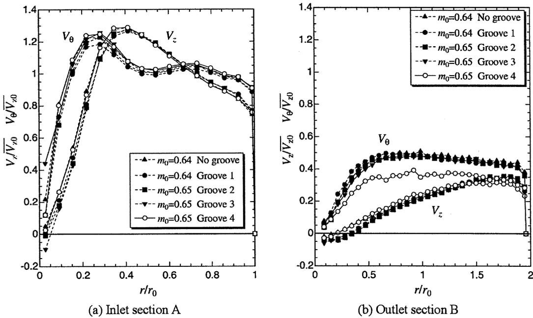
Fig. 4 Velocity distributions in the inlet and outlet sections of diffuser in the case  $m_0 = 0.64$
