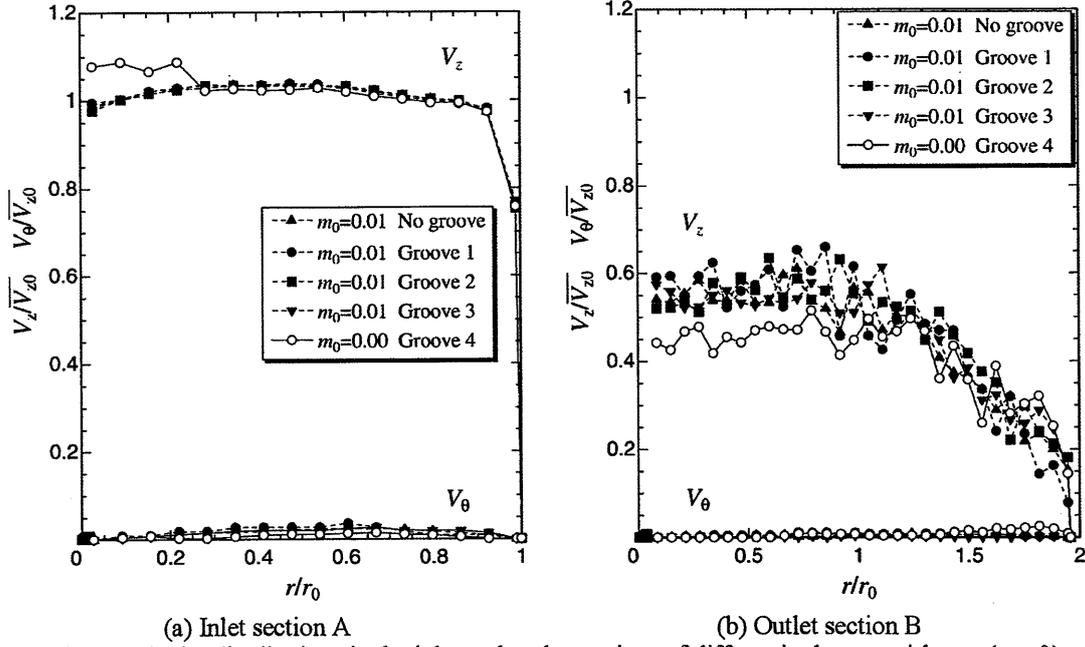
Fig. 2 Velocity distributions in the inlet and outlet sections of diffuser in the no swirl case ( $m_0=0$ )
