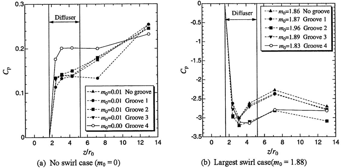
Fig. 9 Static Pressure distribution on the channel wall
