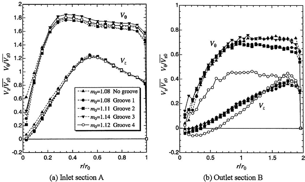
Fig. 5 Velocity distributions in the inlet and outlet sections of diffuser in the case  $m_0 = 1.10$
