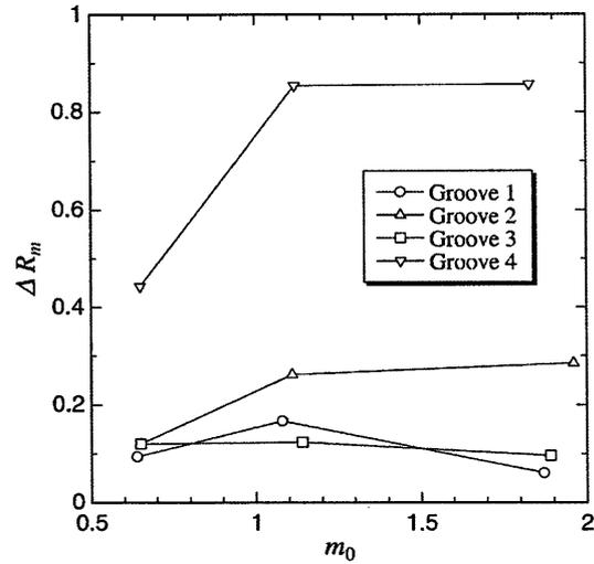
Fig. 11 Change of swirl parameter by J-groove
