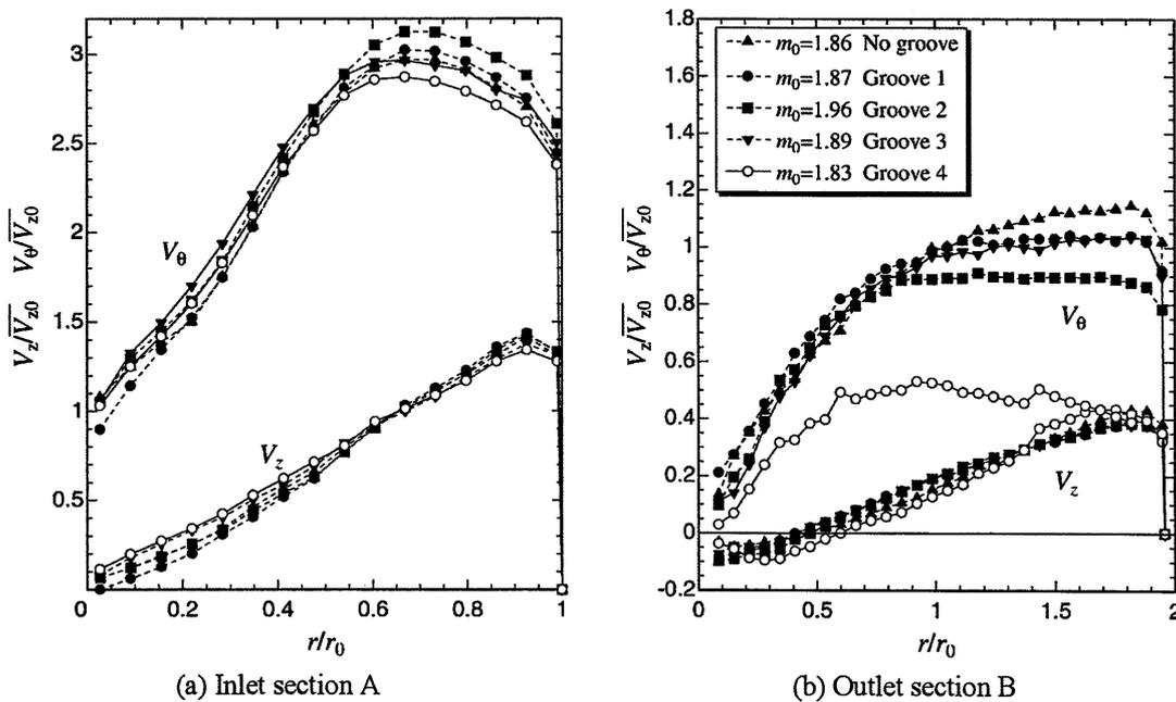
Fig. 6 Velocity distributions in the inlet and outlet sections of diffuser in the case  $m_0 = 1.88$
