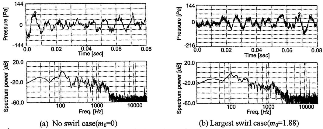
Fig. 3 Pressure fluctuation in the outlet section B in the case of no groove
