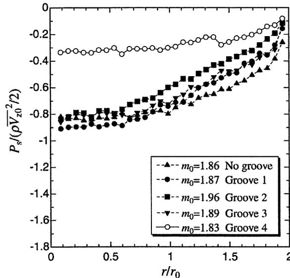
Fig. 7 Static pressure distribution in the outlet section ( $m_0 = 1.88$ )
