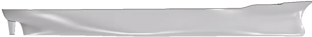
FIGURE 3.1 Geometric model of the S175 containership with a rudder
