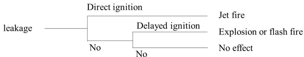
Fig. 3 Hydrogen leakage event tree
