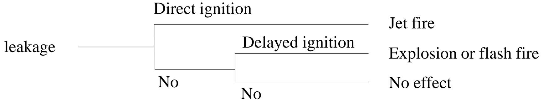
Fig. 3: Hydrogen leakage event tree
