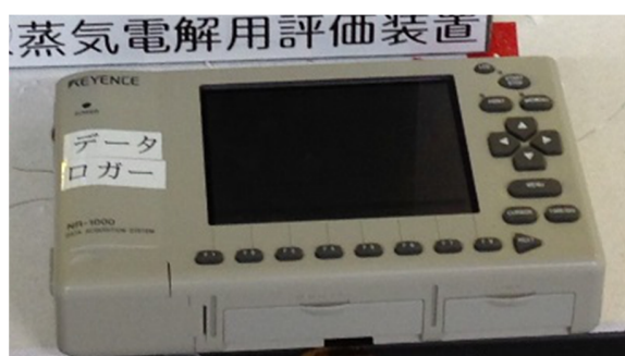
Fig. 2.15 Data logger (NR-1000, Keyence inc., JP)
