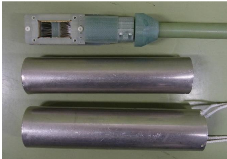
(c) Magnetic shield and end of the probe
